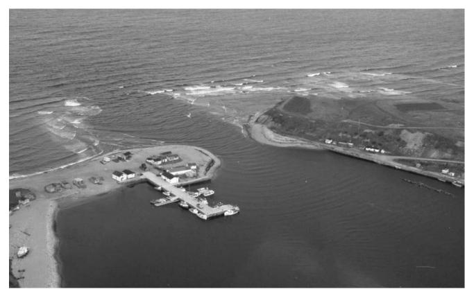
of 6 feet (1.9 m) alongside a 66 foot (20 m) long outer end. Floating wharves are moored on the north and south sides of the Public wharf. A fish plant and bait depot are located at the inner end of the Public wharf. An outflow from the adjacent river is reported alongside the Public wharf.
