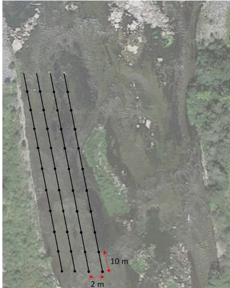
Figure 2. Schematic diagram of transect-based electrofishing sampling design: 40 transects of 10 x 1 m each were placed in a series along the length of the river running parallel to the shoreline, separated by 2 m widths across the channel. Configuration varied depending on sampleable habitat. Points represent the start of a transect. Image is not to scale.
