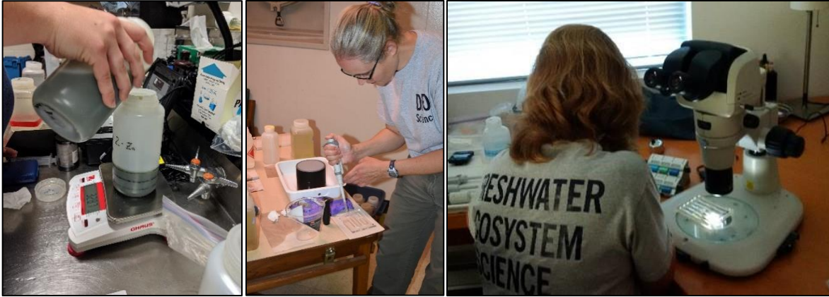
Figure 4. Preparing and analyzing samples for the \geq 50 \mu\text{m} organism size class by splitting the sample for analysis by microscopy (left), transferring aliquots of the sample to a Modified Bogorov counting chamber (center), and counting organisms under a microscope.
