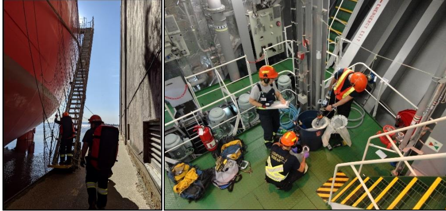
Figure 2. Ballast water sampling team boarding a ship (left) and sampling ballast water in a ship's engine room (right).
