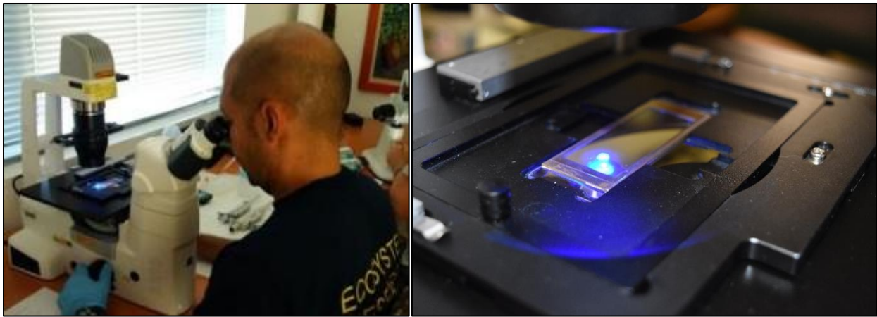
Figure 5. Analyzing samples for the 10 - 50 \mu\text{m} organism size class (left) by counting six 1 mL subsamples on a Sedgewick-Rafter counting chamber under a microscope (right).
