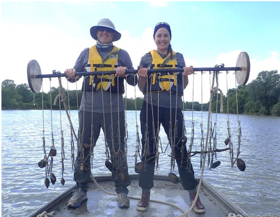
Figure 1. Samplers holding the brail trawl used to sample mussels in non-wadeable habitats.
