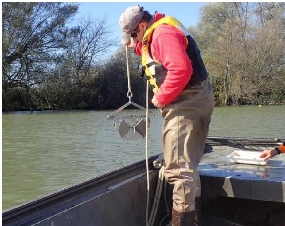
Figure 4. Deploying the Petite Ponar™ benthic grab to collect riverbed material.
