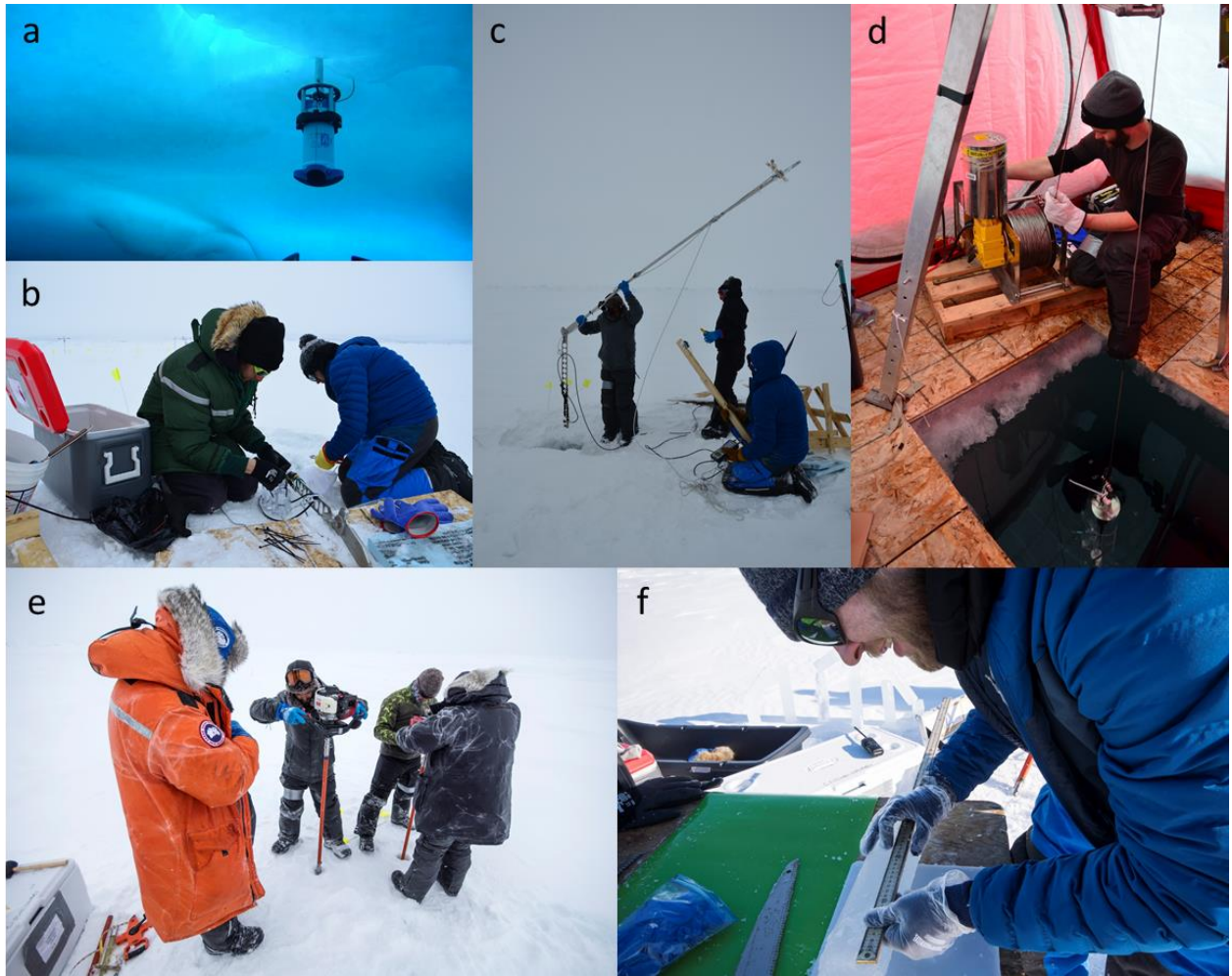
Figure 3. Sampling during the Multidisciplinary Arctic Program (MAP) – Last Ice field campaign, spring 2018. a) ADCP mooring, b) Preparation for primary production incubations, c) Under-ice arm deployment for under-ice light measurement, d) CTD cast, e) MYI coring, f) Measurement of an ice core for core sectioning. Credits: a) C. Katlein, AWI; b to d) DFO, S. Duerksen; e to f) DFO, P. Coupel.
