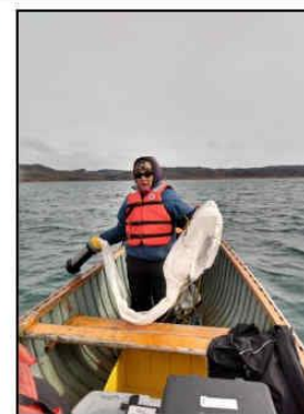
Oloosie using a plankton net to sample water column
