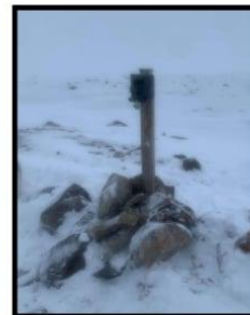
A time-lapse camera was set up in October, 2020 to monitor ice freeze up and break up.
