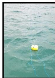
Moorings placed in the water to monitor temperature and saltiness.
