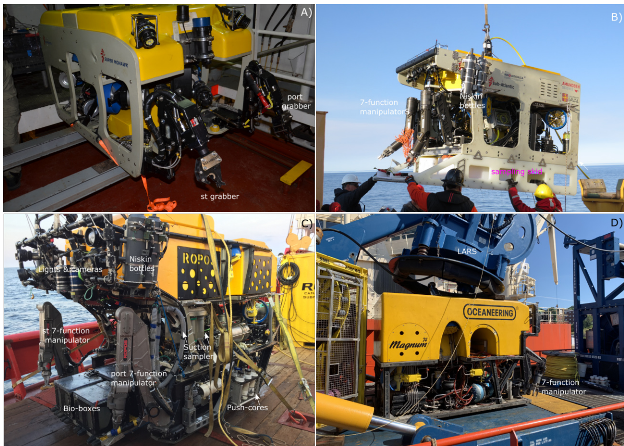
Figure 1. Examples of ROVs used in science. A) Super Mohawk (SuMo) ROV used aboard CCGS Amundsen until 2018 (photo taken in 2014 before adding sampling skid), B) ASTRID, a Comanche ROV currently used aboard CCGS Amundsen , C) ROPOS ROV in 2017 aboard CCGS Martha L. Black , but used internationally, and D) Magnum ROV aboard MV Atlantic Condor in 2022, showing its Launch and Recovery System (LARS).
