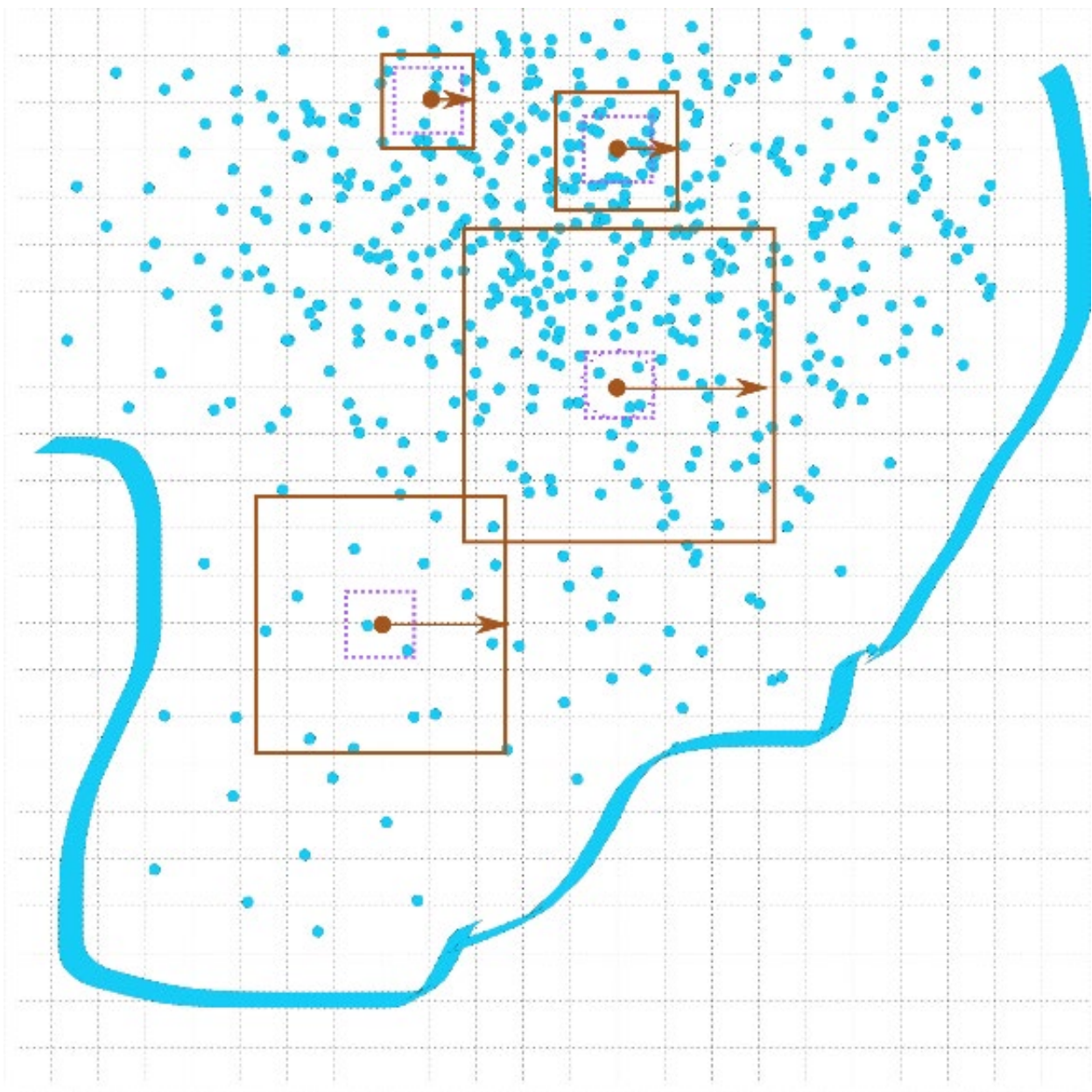
Figure 9. Spatial distribution of data (blue dots) overlaid by a statistical grid. The m nodes represent the centers of each local subdomain S_m which extends to a distance (right-facing arrows; solid squares) that varies depending upon the underlying spatial variability of the data, defined as the distance at which the spatial autocorrelation drops to some small value (e.g., \rho_s = 0.1 ). Data within this distance and parameters obtained from the local analysis are, under the assumption of second order stationarity, used to complete the local model of the spatial or spatiotemporal processes and then predict/interpolate to some fraction of the distance between statistical grid nodes (stippled square). Every statistical node is visited for spatiotemporal modelling. Any overlapping predictions are locally averaged (weighted by number of predictions and prediction variance). As grid size decreases the number of computations increase while reducing computational load and RAM requirements, however, the utility of the model also declines due to small sample sizes entering analyses. Judicious choice of statistical grid density as well as maximum and minimum number of data points and upper and lower bounds of spatial bounds must be balanced.
