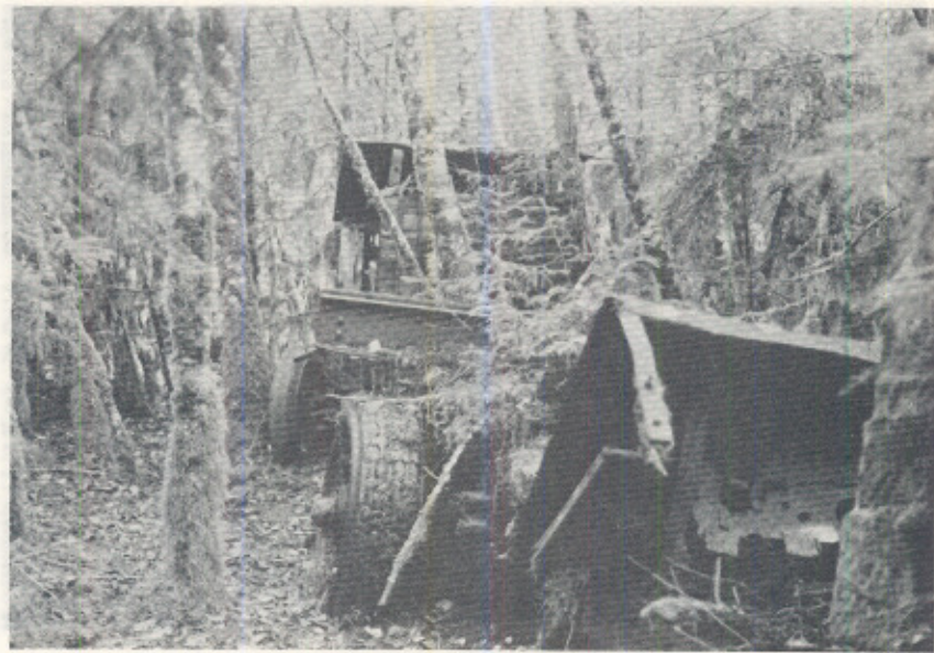
Figure 7: One of the many British Leyland or White logging trucks left at the Mathers logging camp site on Cumshewa Inlet. Note solid rubber tires.
