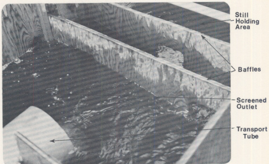
Plate 3: Interior of live box illustrating the staggered baffle arrangement which reduces turbulence and provides a sheltered holding region.
