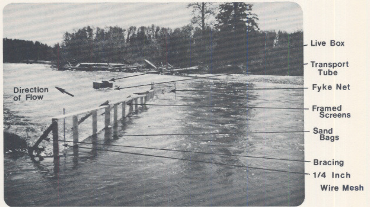
Plate 1: Modified fyke net installation, Seebach Creek, May 22, 1977.
