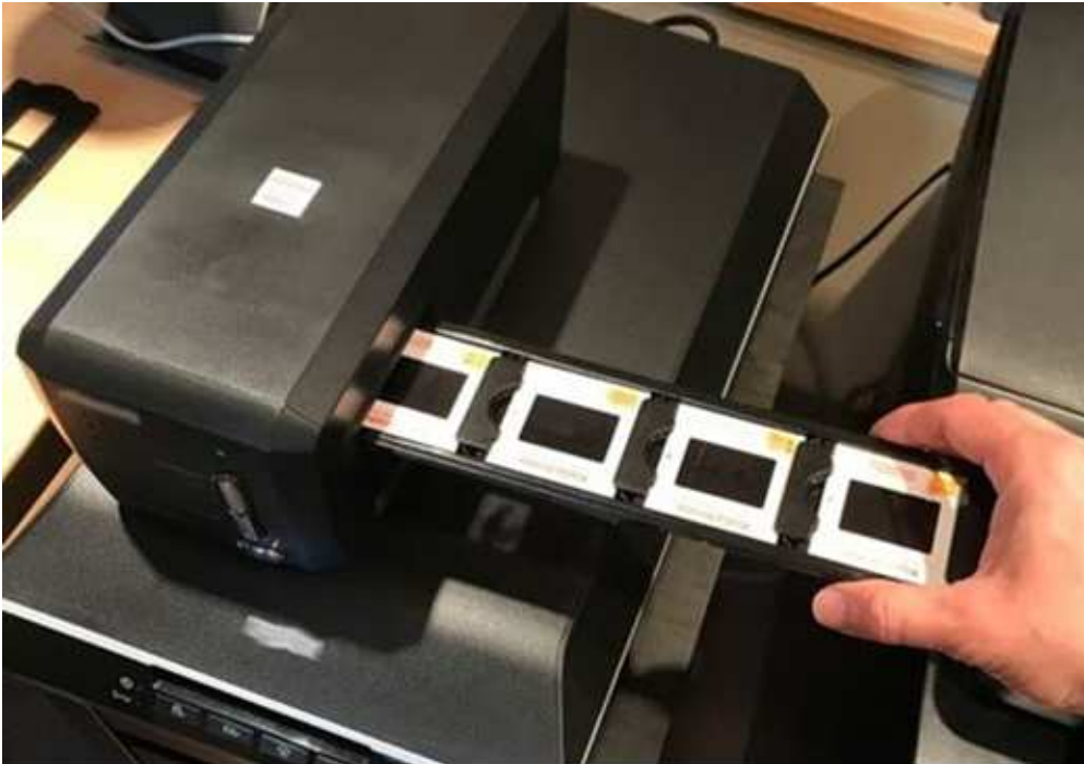
© Government of Canada, Canadian Heritage Information Network. 133977-0012 Figure 10. Loading a slide tray into the CCD scanner.
