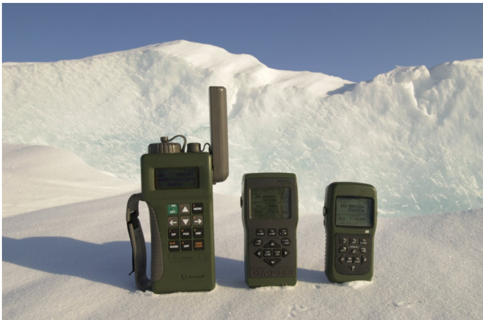
Figure 58: The three GPS receivers tested at CFS Alert. From left to right: the PLGR that had been the previous unit of choice; the PLGR-3, an interim design of the DAGR; and the model that was eventually chosen as the CF's handheld receiver. Photo credit: Janice Lang, DRDC – Ottawa Research Centre.
