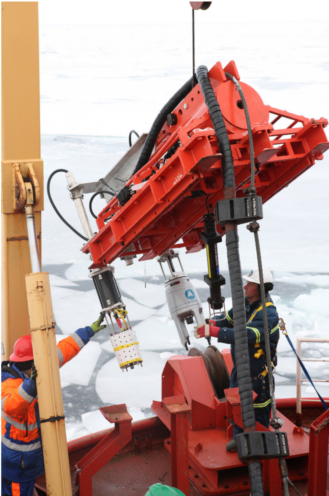
Figure 161: All of the deployed equipment had to be mounted on a very heavy sled that was towed at the stern of the LOUIS. Photo credit: Don Glencross.
