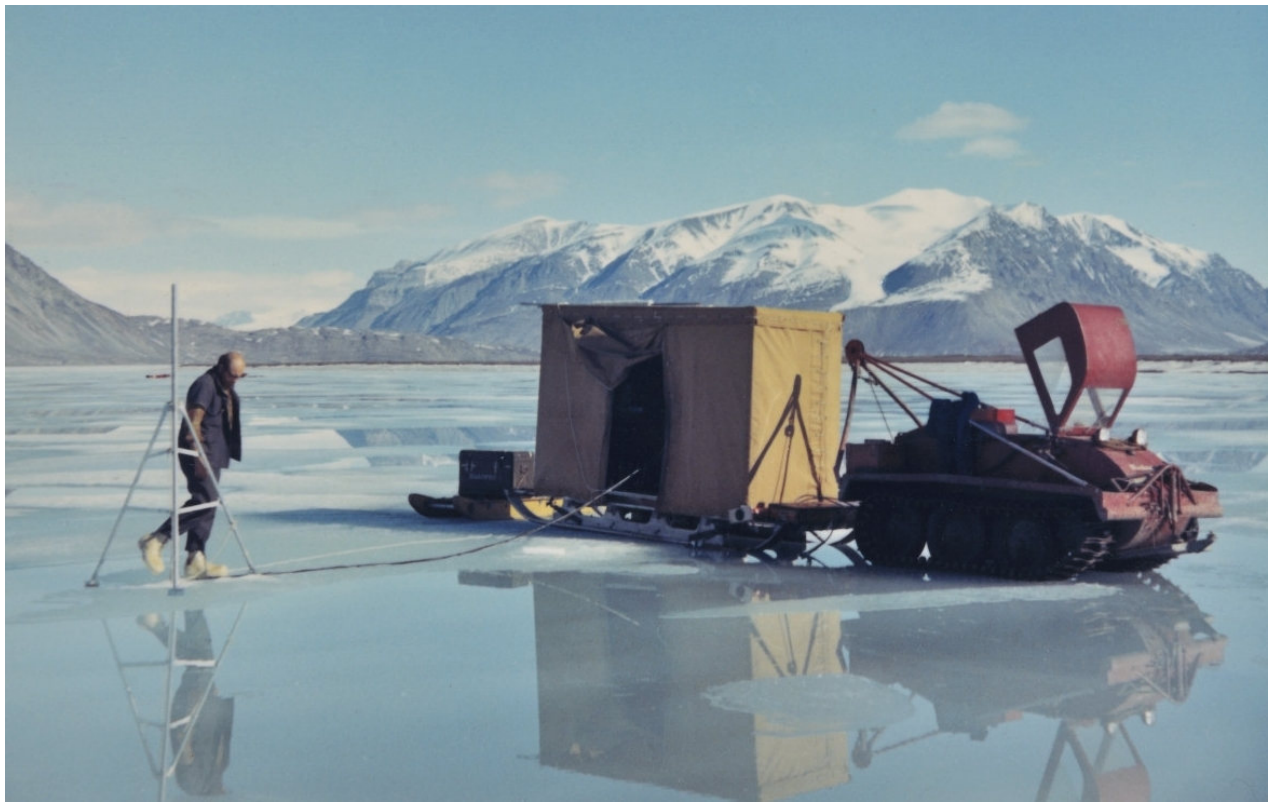
Figure 13: Measuring solar radiation below the ice with a spectrophotometer. Tanquary Fiord, June 1971. Photo credit: Harold Serson.
