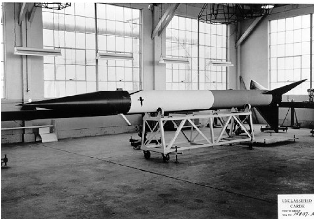
Figure 122: The Black Brant II rocket, developed by CARDE and Bristol Aerospace, was used extensively at Fort Churchill to probe the ionosphere. Photo credit: DRDC.
