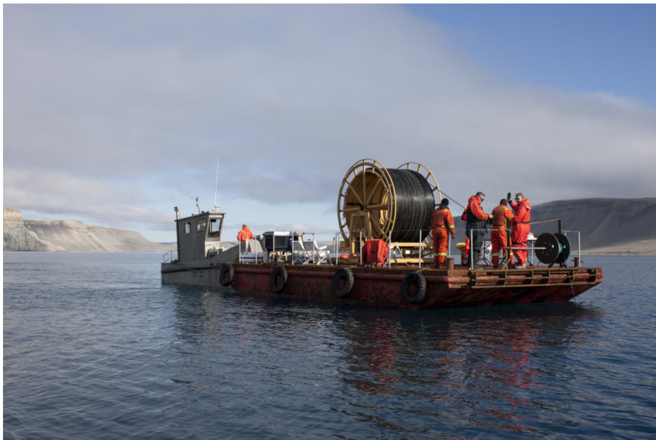
Figure 145: A Coast Guard unpowered barge (known as a “dumb barge”) carrying a large powered reel is used to recover the telemetry cable. The barge is propelled by a motorized shore-patrol barge. Photo credit: Dan Hutt, DRDC – Atlantic Research Centre.
