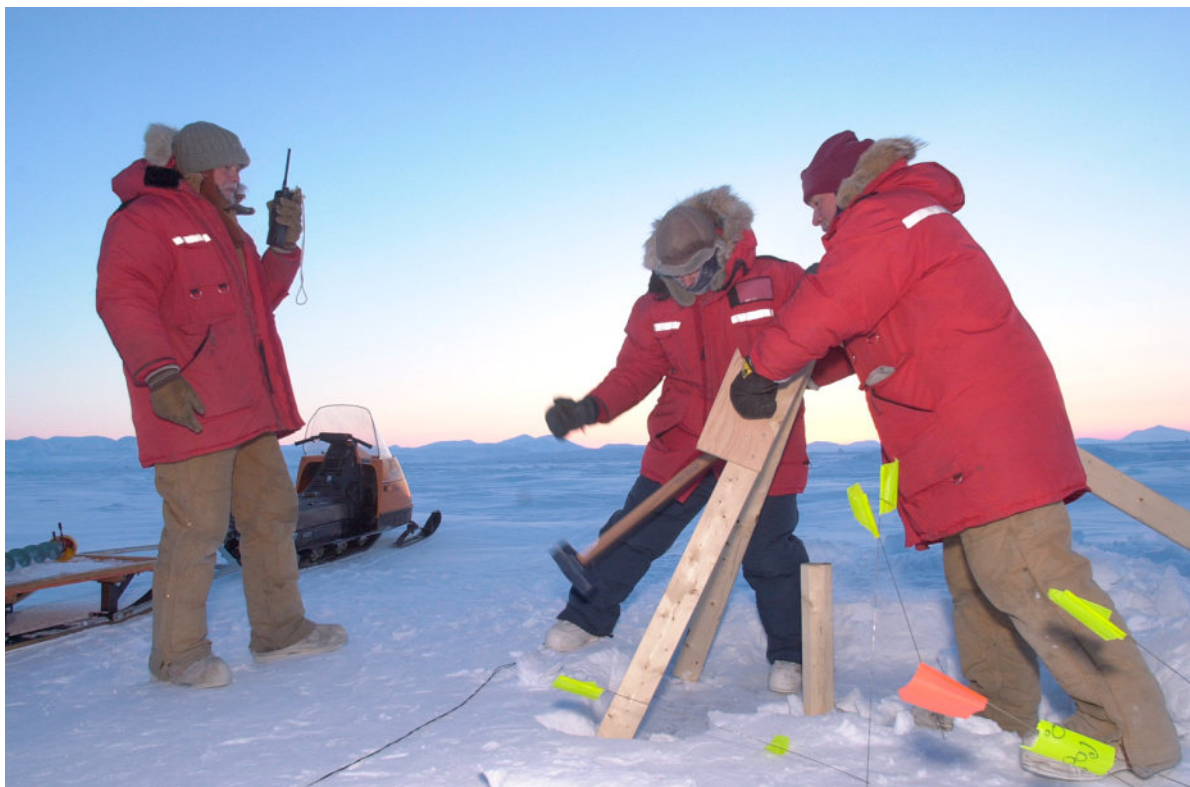
Figure 59: Ron Verrall, Stan Dosso, and Don Richard create seismic waves in the ice with the Hammer Source. Photo credit: Janice Lang, DRDC – Ottawa Research Centre.
