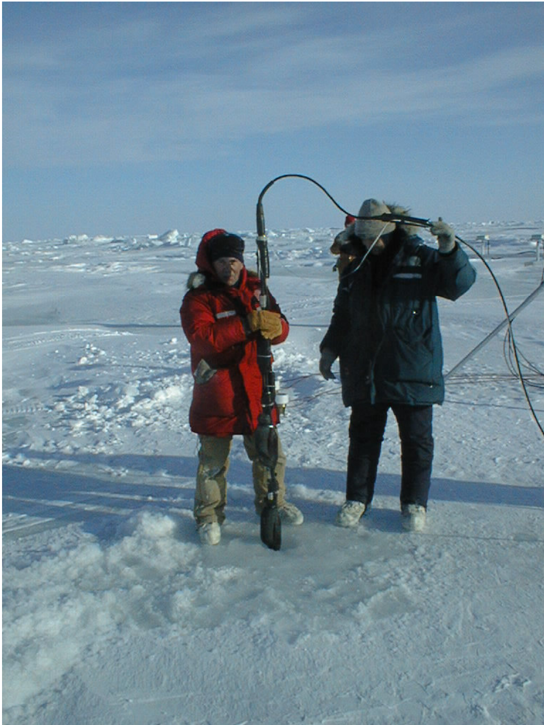
Figure 139: Don Richard and Mel MacKenzie are shown with an early version of an acoustic array built using the developing RDS digital array technology. They are in the process of deploying the array through a 6-inch diameter hole in the ice. Photo credit: Garry Heard.
