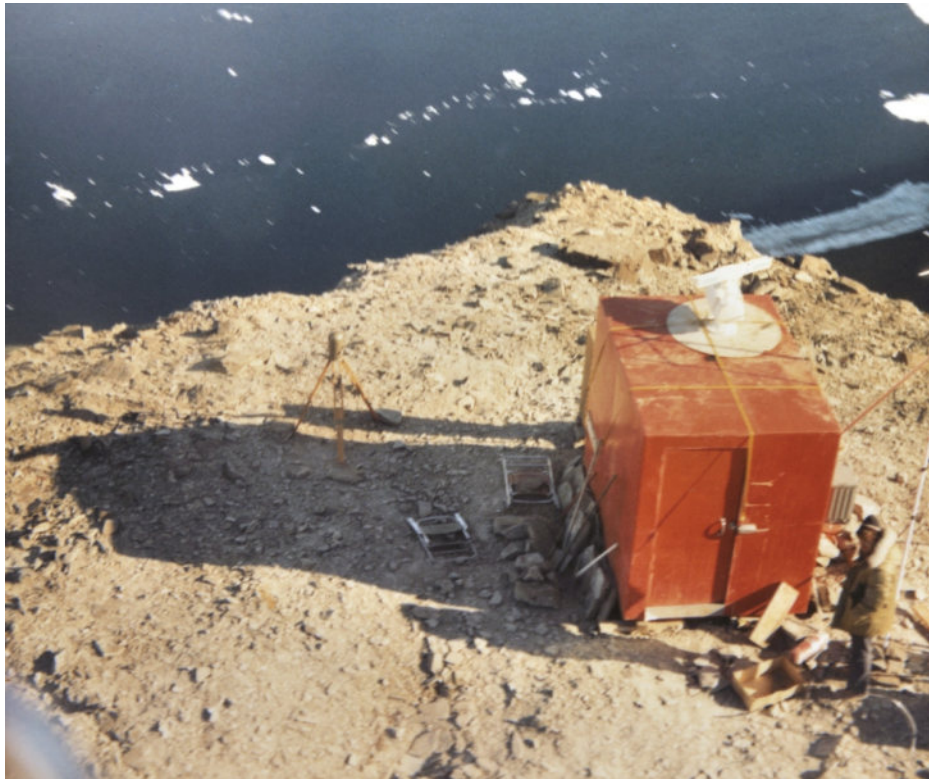
Figure 50: Looking down on the radar shack (with antenna on top). It is about four metres away from the cliff edge. Photo credit: DRDC – Ottawa Research Centre.
