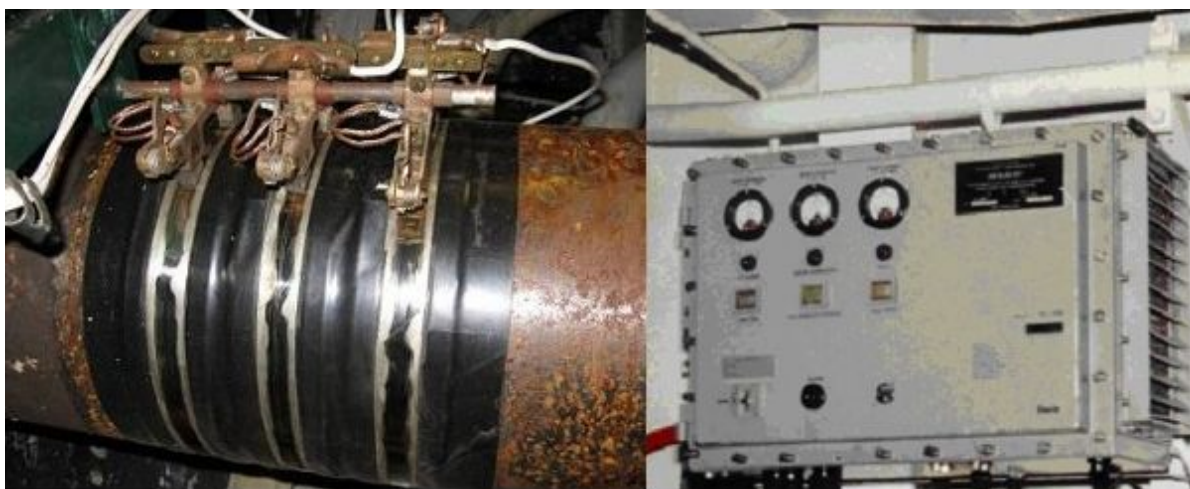
Figure 114: A modern ASG system originating from Arctic research. The left-hand picture shows slip-rings, and the right-hand picture shows the control box. Photo credit: DRDC.
