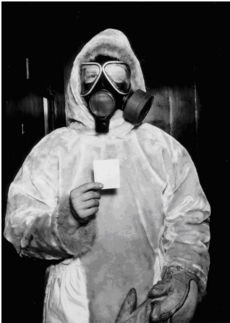
Figure 48: Testing a new nylon pile fabric in the DREO cold chamber, which could be cooled to -40^{\circ}\text{C} . They are also giving a cold weather test to a gas mask (or respirator). Photo credit: DRDC – Ottawa Research Centre.
