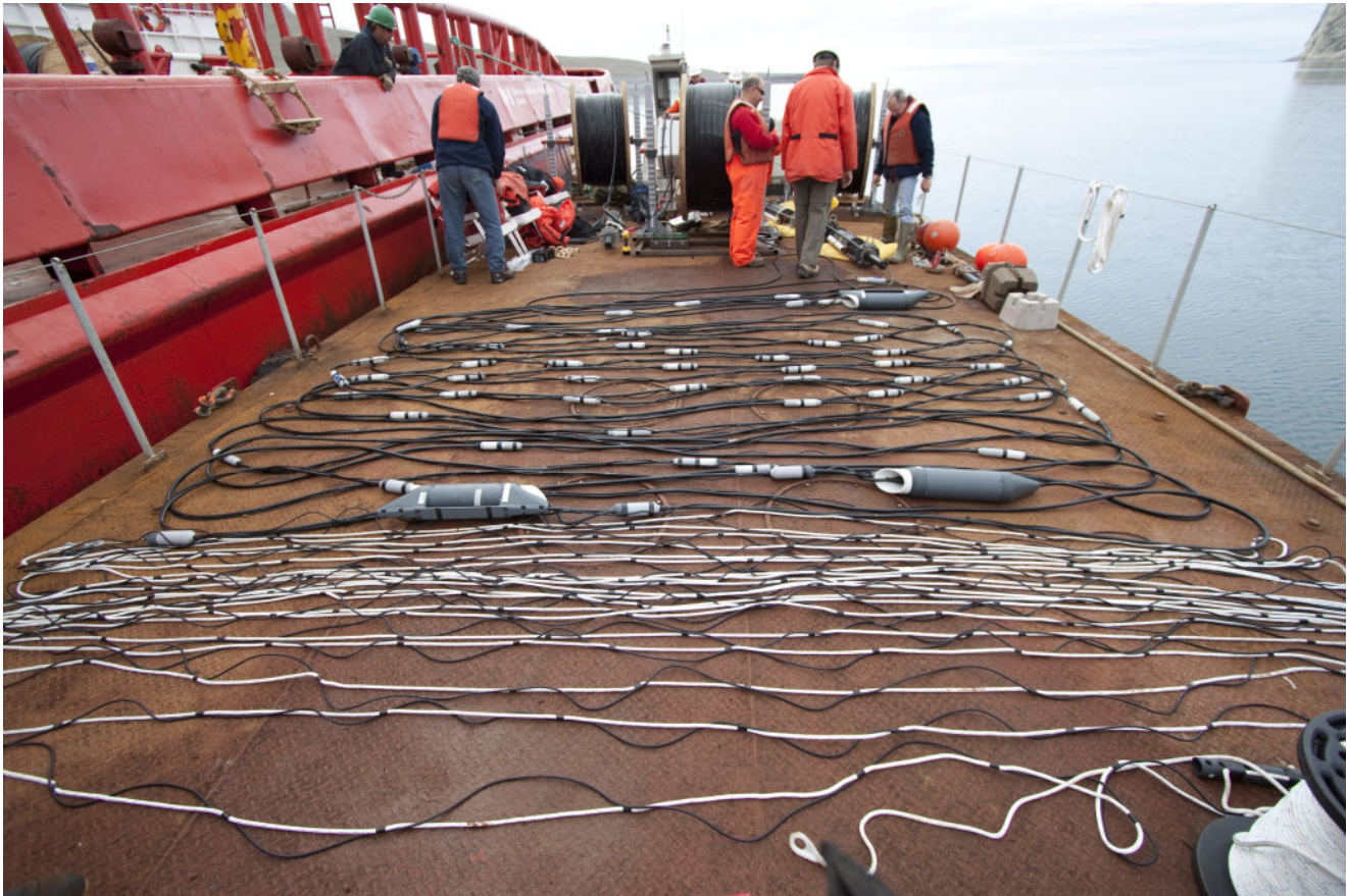
Figure 146: A first generation Northern Watch array is shown laid out on the deck of the barge. The cable reels hold the telemetry cable that transmits the array data to shore. Photo credit: Dan Hutt.
