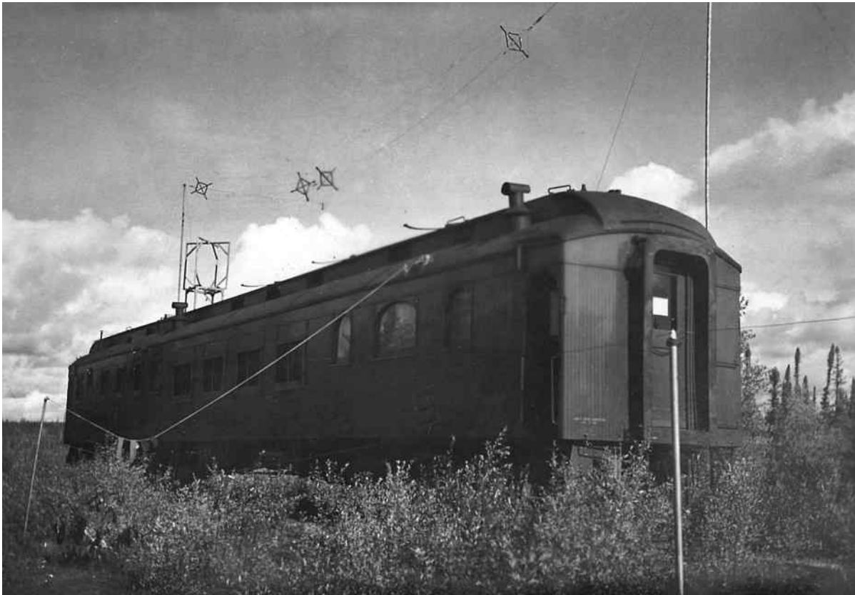
Figure 20: A mobile ionosphere experiment. The railway carriage that contained the laboratory was left on a Hudson Bay Railway siding for several days at a time. Note the antennas on top of the carriage. What looks to be an antenna off to the left of the car is probably just a clothesline. Photo credit: Harold Serson Collection, DRDC – Ottawa Research Centre.
