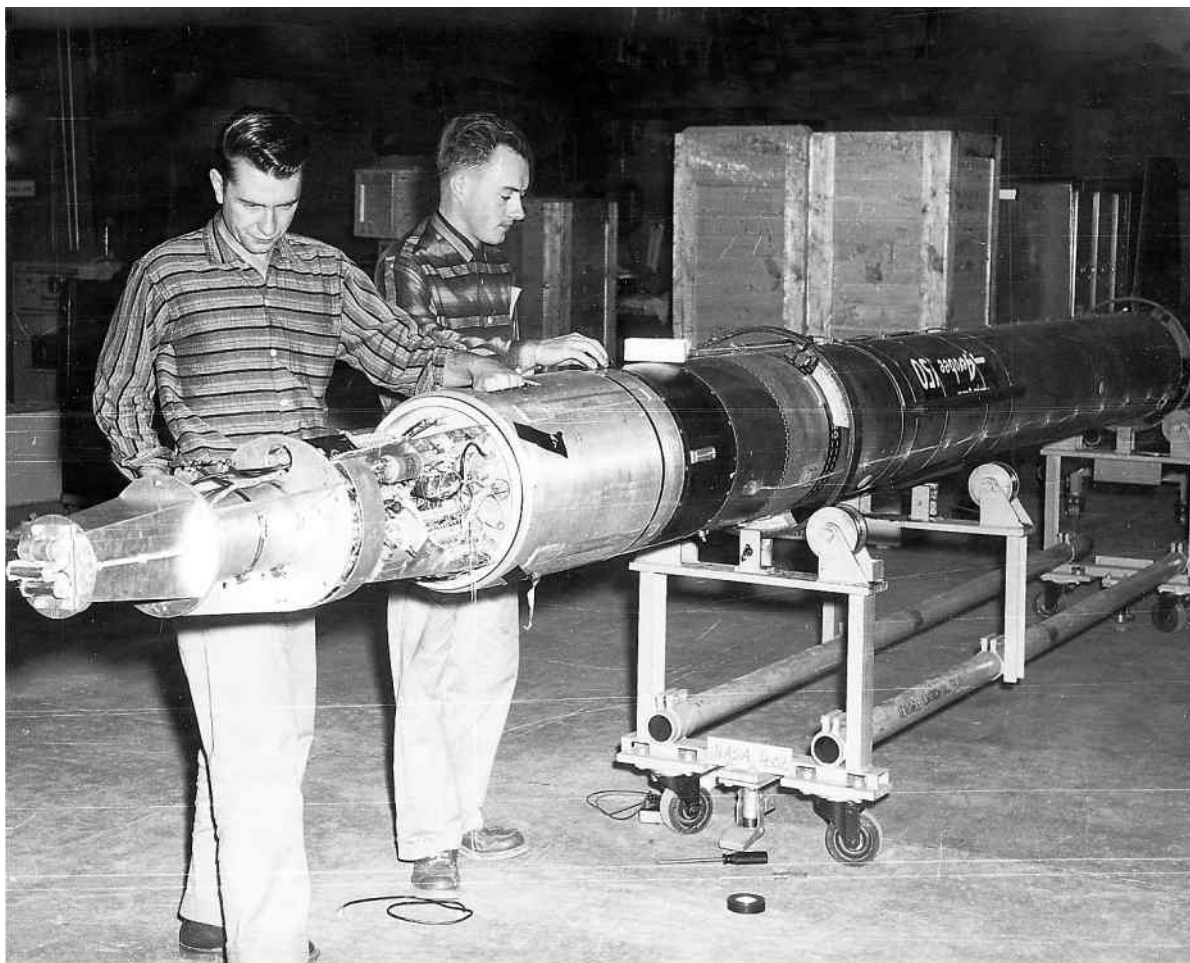
Figure 24: The first DRTE rocket payload was launched at Churchill in 1959 by an Aerobee 150 rocket provided by NASA. Steve Cebuliak and Gordon Bird inspect the instruments. Photo credit: NRC. The print was provided by Stu McCormick who manages the following website: http://www.friendsofrcrc.ca/Projects/Sounding%20Rockets/rocket.html .
