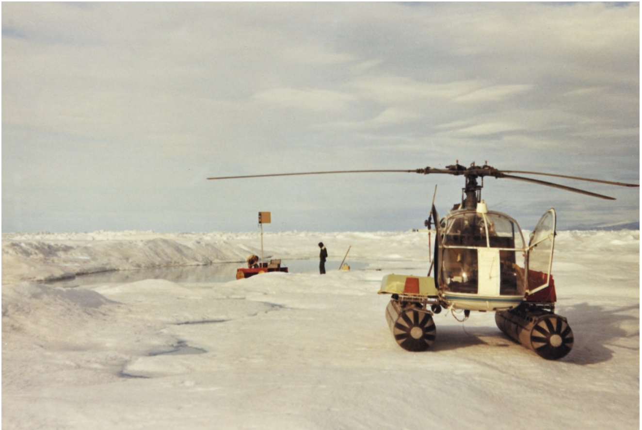
Figure 52: Setting out an ice station complete with radar transponder, anemometer, and current meters. Note the open water in the melt hole. Unfortunately these holes were rare. Moreover, the hole had to be adjacent to ice thick enough to take the weight of the helicopter. Photo credit: DRDC – Ottawa Research Centre.
