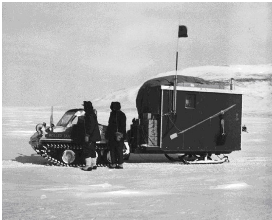
Figure 66: John O'Malia and Carl Kelly with Bombardier J5 tractor and sled. The small building on the sled is known as a "Wannigan." Photo credit: DRDC.
