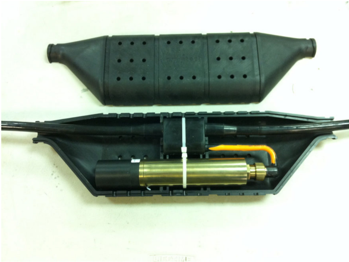
Figure 147: A second generation Northern Watch hydrophone assembly. The orange cable breakout is the same material as the black cable covering. The blending of colours at the interface points shows how the materials mix to create a continuous covering. Photo credit: Don Glencross.
