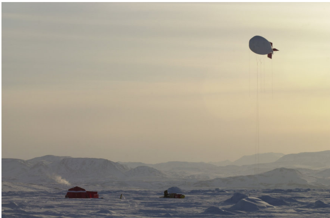
Figure 55: Icecamp southeast of King William Island (NU) with the kytoon floating overhead. The kytoon would lift the icepicks to a height of approximately 210 m and, upon radio command, drop them. Photo credit: Janice Lang, DRDC – Ottawa Research Centre.
