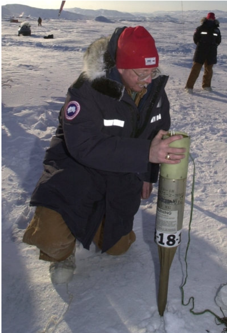
Figure 54: Geobuoy being held by Mike Vinnins. The “prong” is made of bronze-steel. Ordinary steel that size bends upon impact. Photo credit: Janice Lang, DRDC – Ottawa Research Centre.
