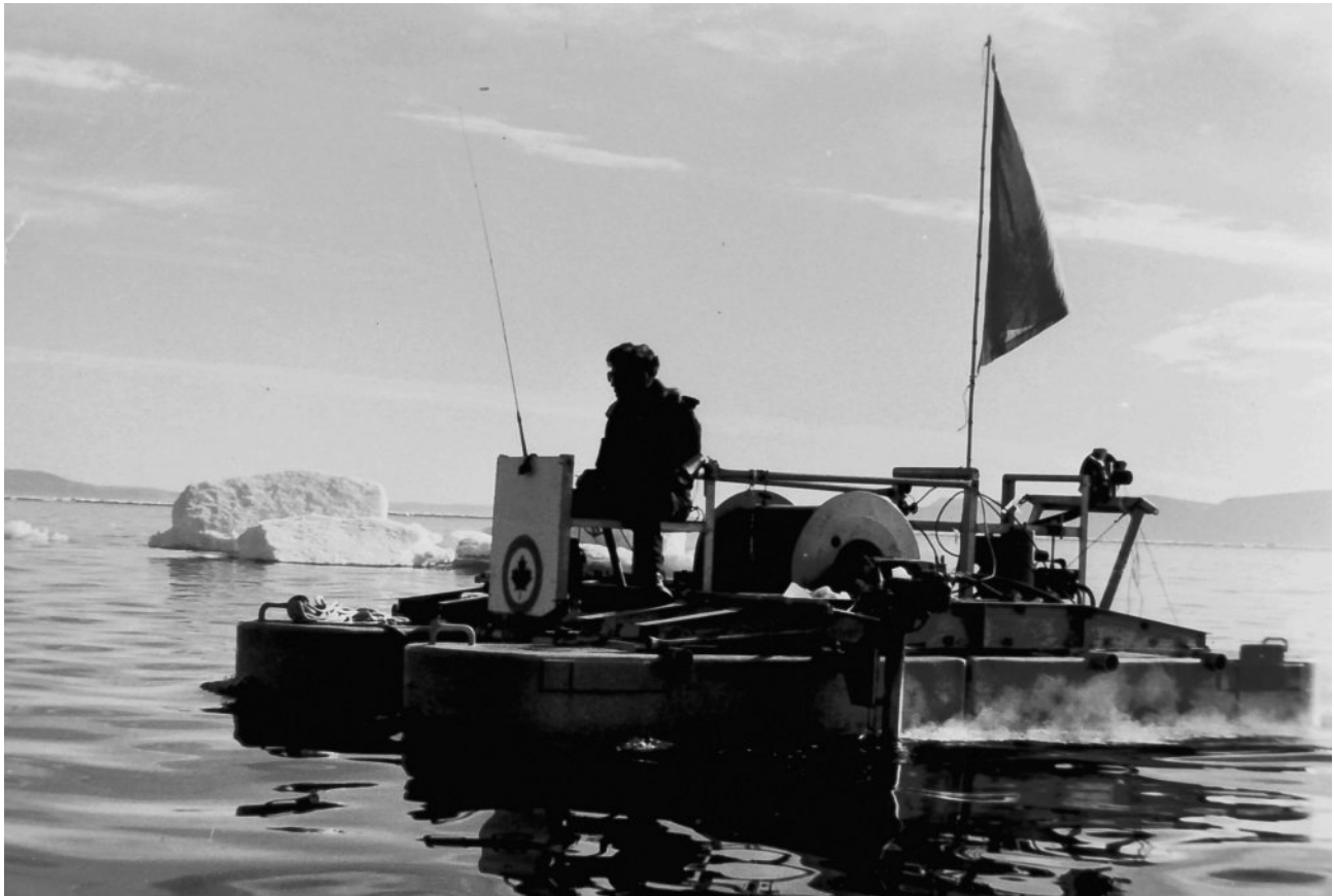
Figure 84: A catamaran was the cable-laying platform. It was light, shallow-drafted, stable, inexpensive, and it had a large working platform—like a raft. It was propelled by two outboard motors. The operator here is Capt Stannard (Stan) Toole, an airforce officer who was seconded to DREP at the time. Photo credit: DRDC.
