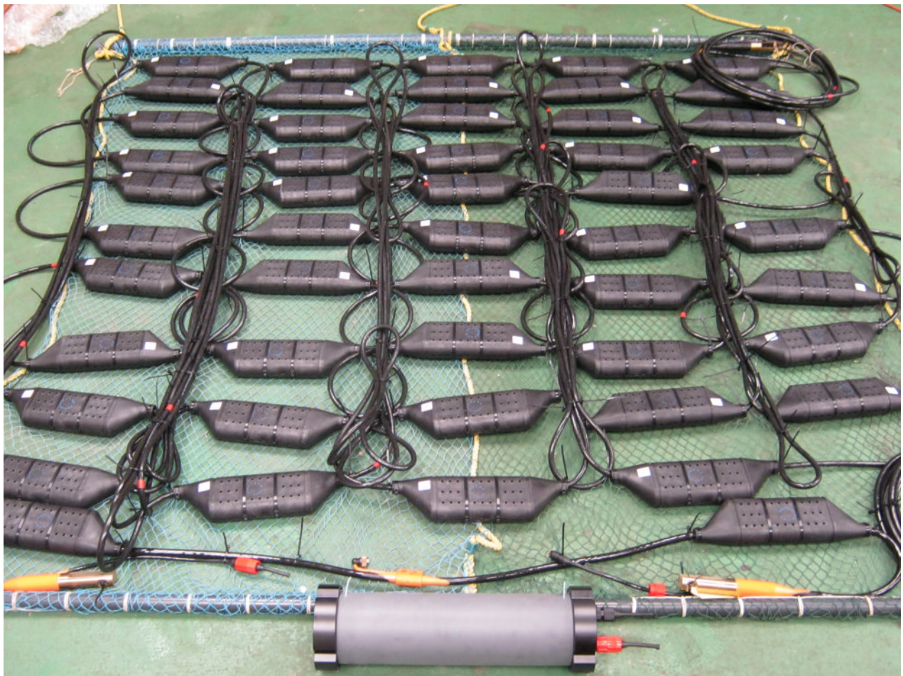
Figure 148: A prototype second generation Northern Watch array ready for testing and calibration at the DRDC Atlantic Calibration Barge Facility. Photo credit: Derek Clark.
