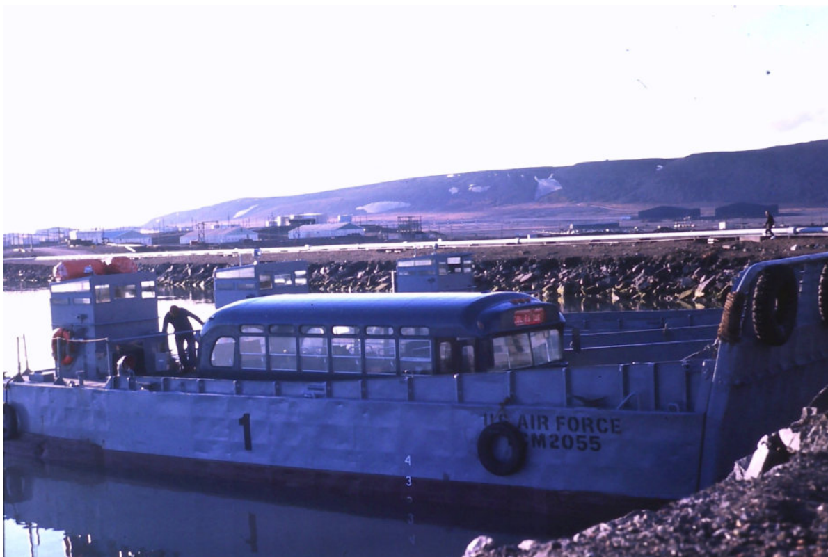
Figure 132: A old bus, missing its engine, was placed on a landing craft and used as a laboratory to conduct measurements in the fiords. Photo credit: C.R. Yool.
