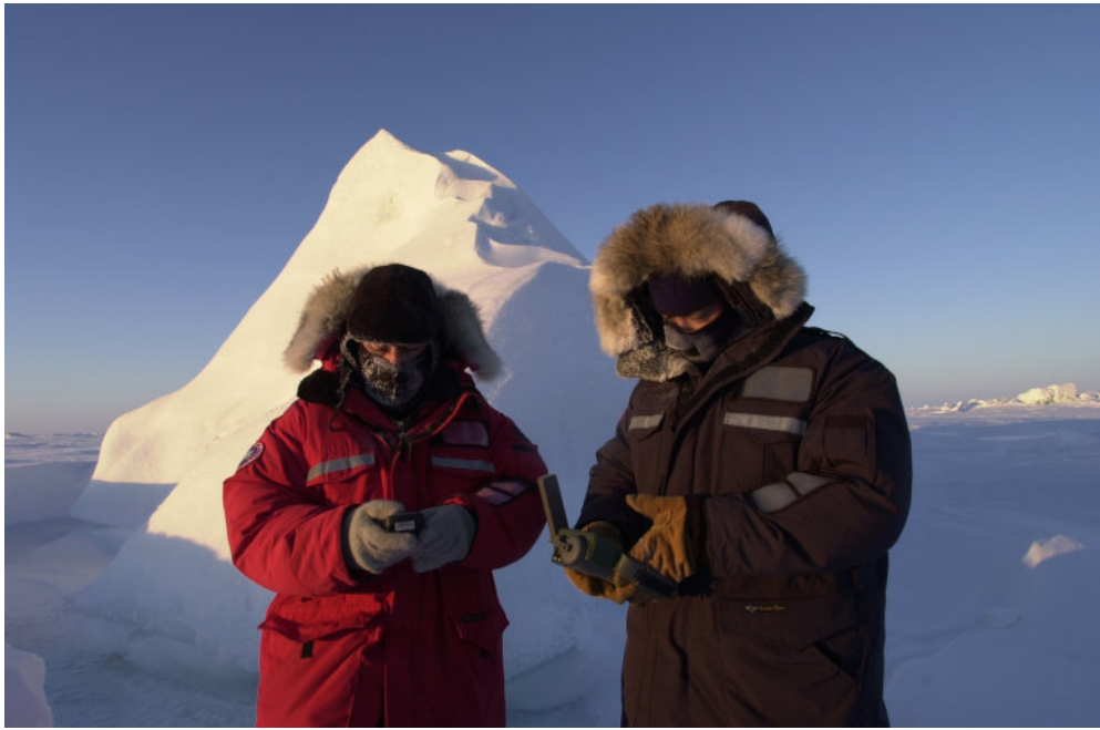
Figure 57: Mike Boyle (DRDC – Ottawa Research Centre) and Capt Clay Koschnik (USAF) cold-testing the DAGR and PLGR (Precision Lightweight GPS Receiver) receivers at CFS Alert. Photo credit: Janice Lang, DRDC – Ottawa Research Centre.
