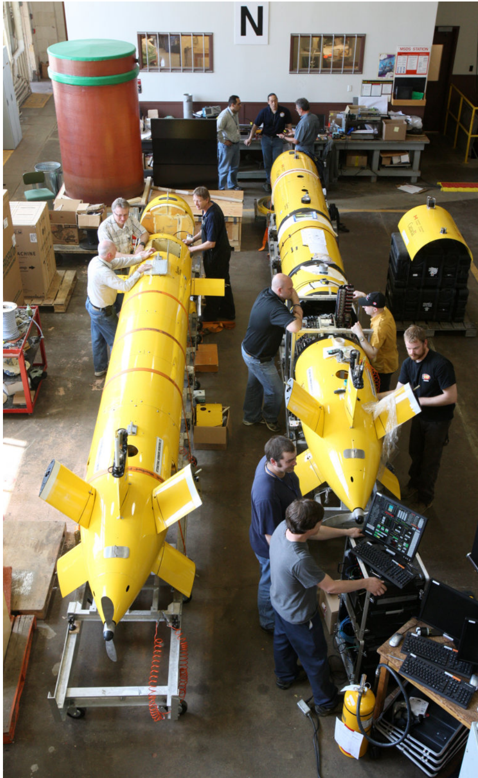
Figure 149: The two modified ISE Explorer AUVs are shown being tested in the Heavy Engine Laboratory at DRDC Atlantic. Various compartments are open, and the modular nature of the AUVs is apparent. Each Explorer breaks down into seven sections to facilitate transport in small boats or aircraft. Photo credit: Don Glencross.
