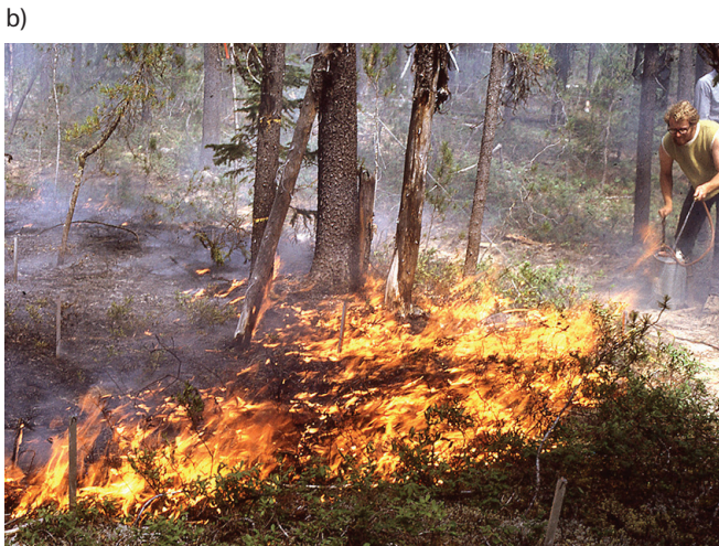
Figure 1. View of (a) flame dimensions perpendicular to the flame front ( L = flame length, D = flame depth, A = flame angle, h = flame height), and (b) of a surface fire flame front (Darwin Lake experimental fire Unit 2, 1974. Head fire intensity 160 kcal/s-m (670 kW/m)).
