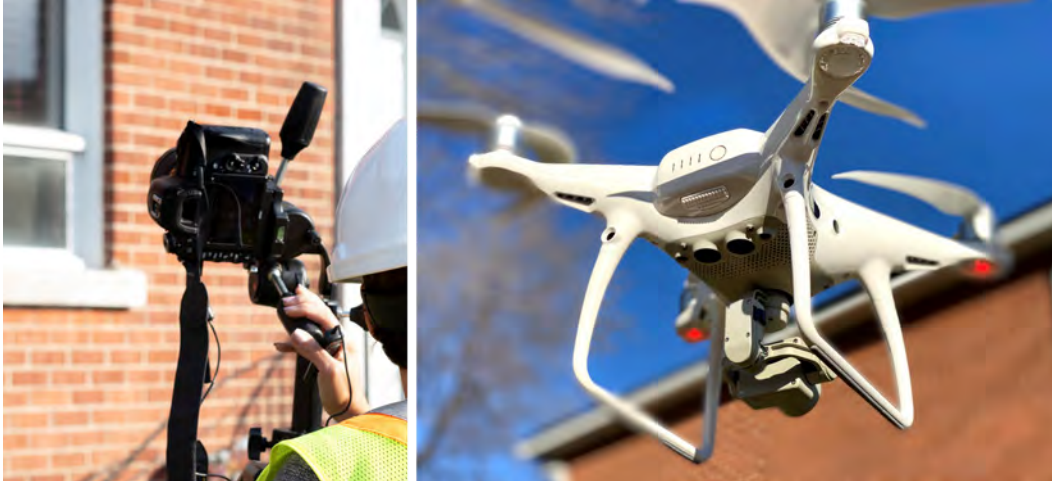
Figure 7-5: Photographic data being captured by digital SLR and by drone for photogrammetry model.
