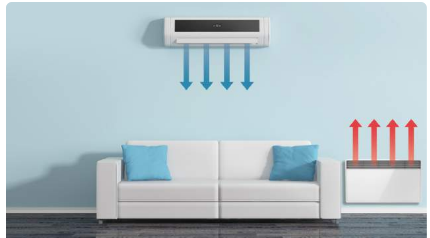
Eliminating simultaneous heating and cooling
