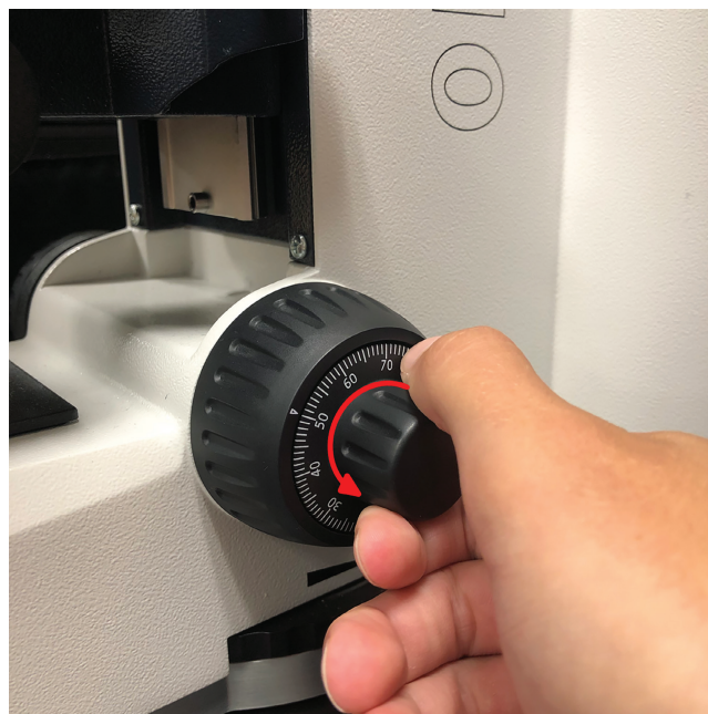
Figure 2. Zeiss Axio Scope microscope fine-focus dial, indicating drive direction for increasing the height of focus. Photograph by C. Greaves. NRCan photo 2022-445
