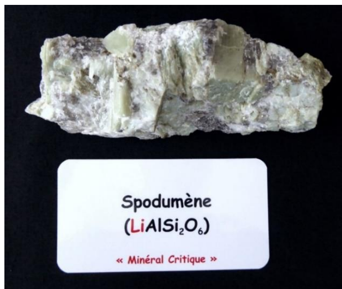
Figure 2.12: Sample of spodumene (light green mineral) from the North American Lithium mining site in La Corne in Abitibi, Quebec (donated by P. Mercier-Langevin).
