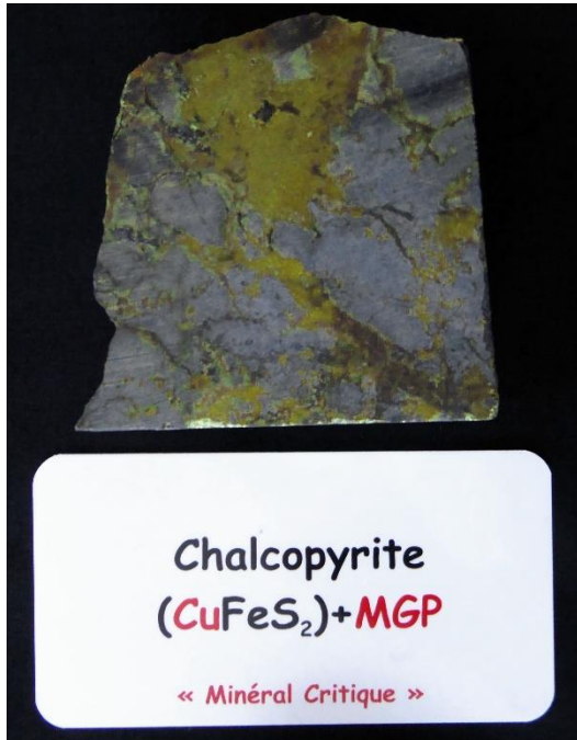
Figure 2.6: Sample of chalcopyrite, a brassy yellow mineral with metallic lustre, from the Rouyn-Noranda area in Abitibi, Quebec (donated by P. Mercier-Langevin).
