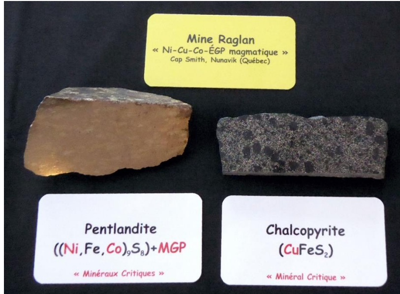
Figure 2.5: Samples of pentlandite and chalcopyrite from magmatic nickel ore taken from the Raglan Mine in the Cape Smith Belt in Nunavik, Quebec (donated by M. Houllé).
