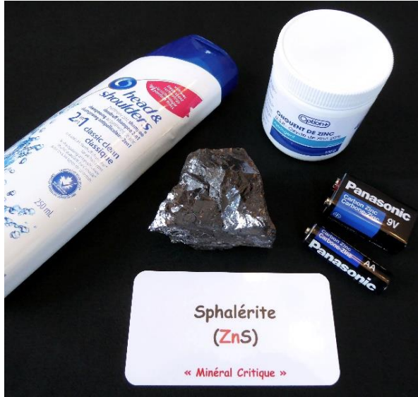
Figure 2.11: Sample of sphalerite (ZnS) from the Chisel North mine, located in Snow Lake, Manitoba (donated by P. Mercier-Langevin) and examples of products that incorporate zinc in their manufacturing process.
