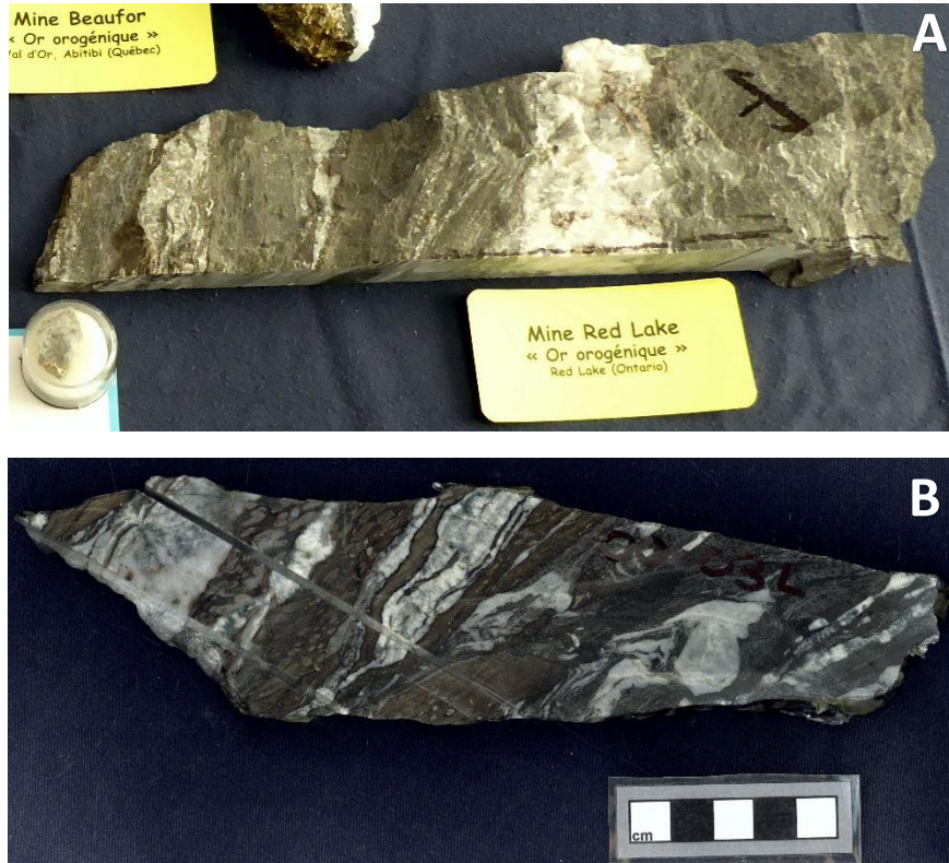
Figure 3.6: Orogenic gold ore samples from the Red Lake Mine in Northern Ontario (donated by B. Dubé).
