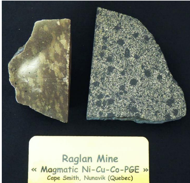
Figure 3.9: Magmatic nickel ore samples from the Raglan mine in the Cape Smith Belt, Nunavik (donated by M. Houlié).
