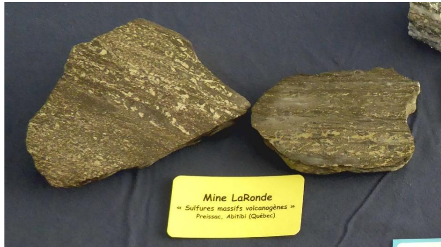
Figure 3.8: Volcanogenic massive sulphide gold-rich samples from the LaRonde Penna mine located in Preissac, Abitibi (don de P. Mercier-Langevin).
