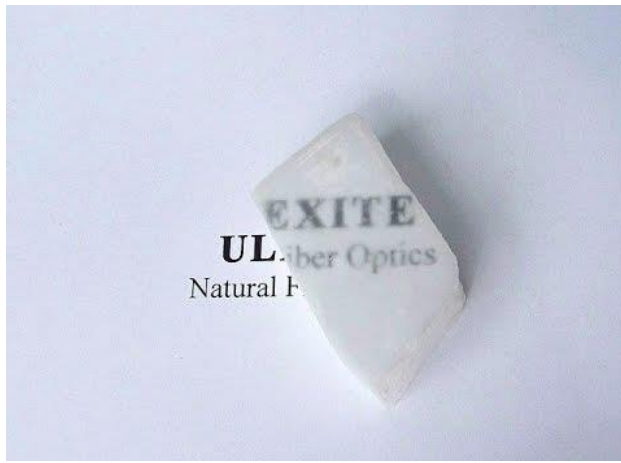
Figure 4.3: Ulexite specimen allowing light propagation
