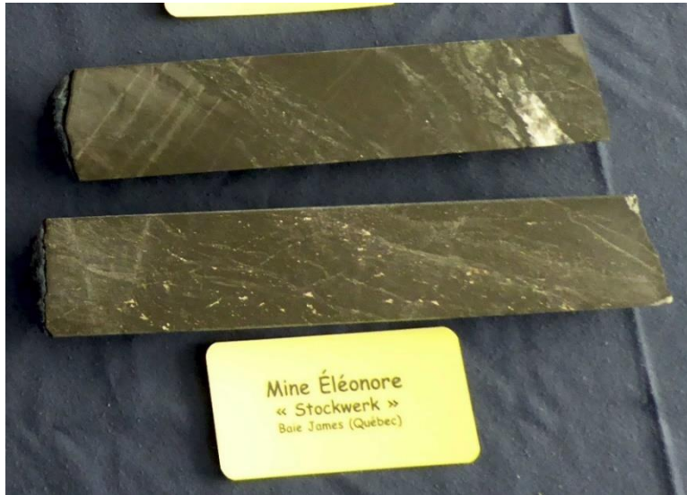
Figure 3.7: Examples of stockwork gold ores from the Eleonore mine in the Eeyou Istchee Baie-James area (donated by A. Fontaine).
