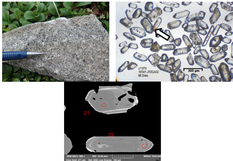
Figure 10: Upper left is a hand sample of 16RAY-JR052A02. Photograph by J.J. Ryan. NRCan photo 2021-532; Upper right is a photomicrograph of zircon grains from the sample. There were very few zircons obtained from the crushing and mineral separation processes so grains were picked directly from the methylene iodide sinks without any magnetic separation steps undertaken; Bottom image is the SEM BSE image of grains 21 and 22 showing homogeneous zircon texture and simple oscillatory zoning.
