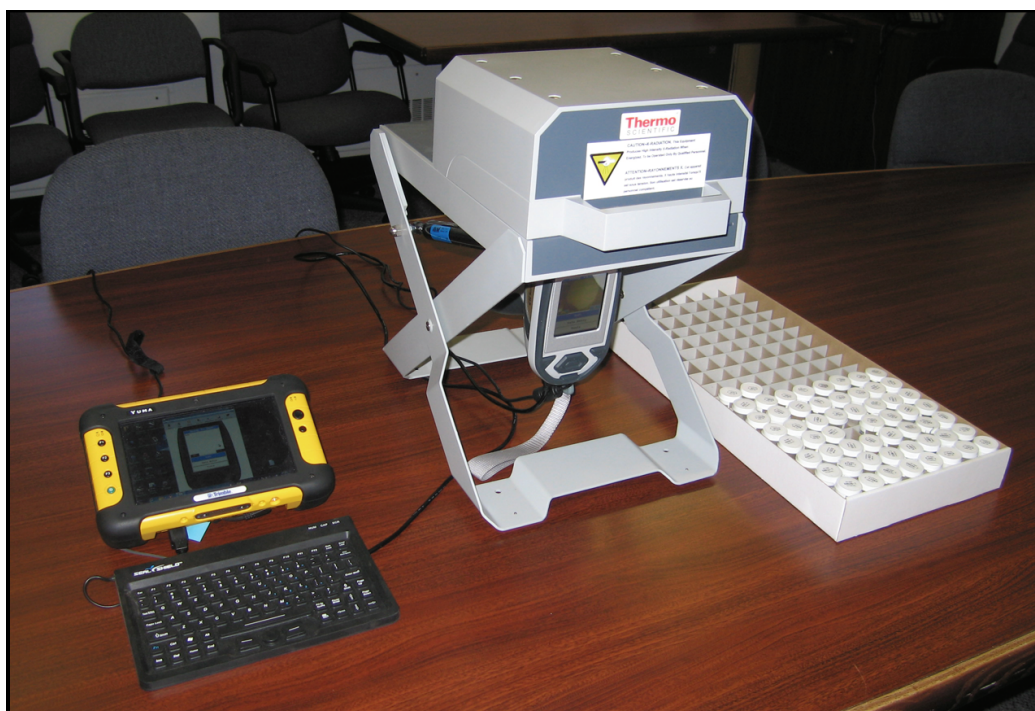
Figure 2. Bench mounted (closed system), pXRF operated via portable computer, with vials of Till-1 and Till-3 samples of vary thickness in a box on the right hand side of the photo. Photograph by R.D. Knight. NRCan photo 2020-926.
