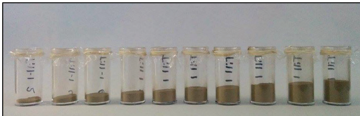
Figure 1: Samples of Till-1 in plastic vials, covered by Chemplex® Prolene® film secured with an elastic band. Samples range from 1 mm thickness (on the left), to 20 mm thickness (on the right). Photograph by A.R.R. Landon-Browne. NRCan photo 2020-937.
