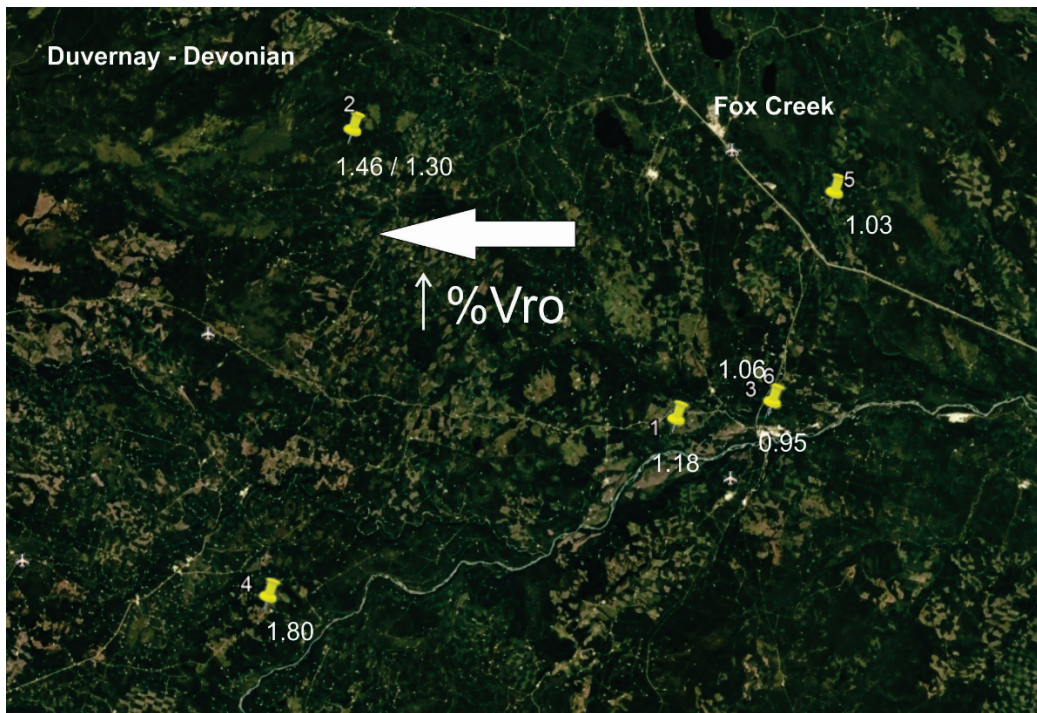
Figure 1.3: Spatial distribution of average %Vro data for the Duvernay Formation in the Fox Creek area. The yellow pins correspond to well locations. For well #2, the first value is the new petrographic data and the second is the vintage data.
