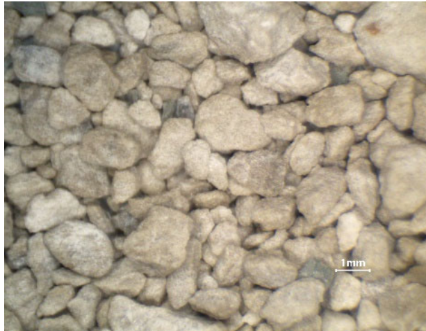
Figure 5-11. Photograph of fine-grained dolostone of Lions Head Formation in drill cuttings from Greenock Township (T002730), at a depth of 424.3 m (1392 ft) (10x magnification). Photo by Candace Freckelton.
