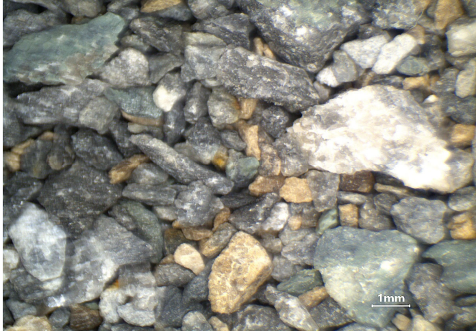
Figure 4-9. Well T000154, sample tray 4980, from 1285 to 1292 feet A-1 Carbonate with green dolomite fragments. Photo by Alexandre Cachunjua.
