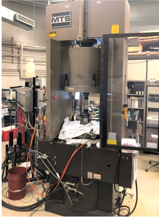
Figure 10. Strength and permeability testing were carried out using the servo-controlled MTS Rock Mechanics Testing System, Model 815. Photograph by S.Gaines. NRCan photo 2021-136.
