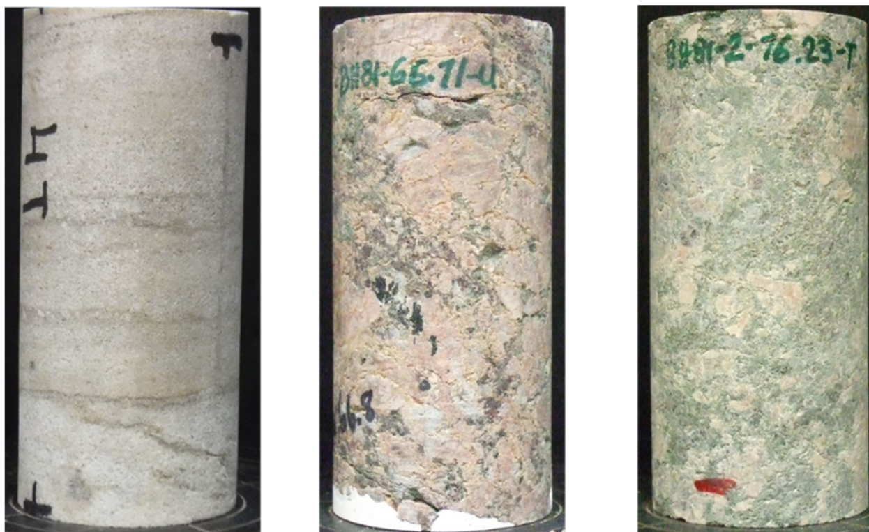
Figure 9. Representative prepared core samples. Left: BC81-2-4T (sandstone, 29.23 m); Centre: BC81-2-66.71-U (weathered granitic gneiss with hydrostone filling on the lower end, 66.71 m); Right: BC81-2-76.23-T (granitic gneiss with chlorite alteration, 76.23 m)
