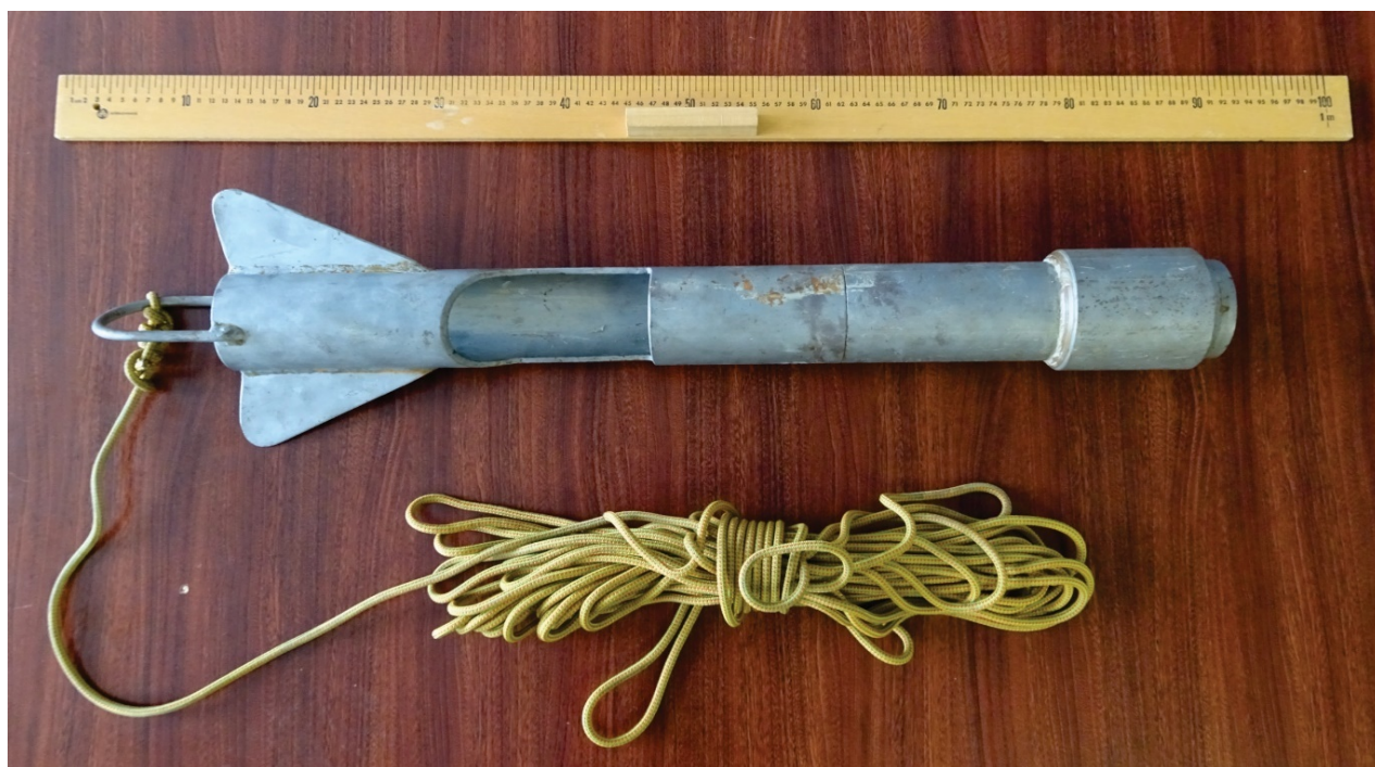
Figure 2 About 1 kg of wet lake sediment ( gyttja ) is collected by dropping the sampler (pictured) from a platform attached to the float of the helicopter (photograph by M.W. McCurdy, NRCan photo 2021-198).
