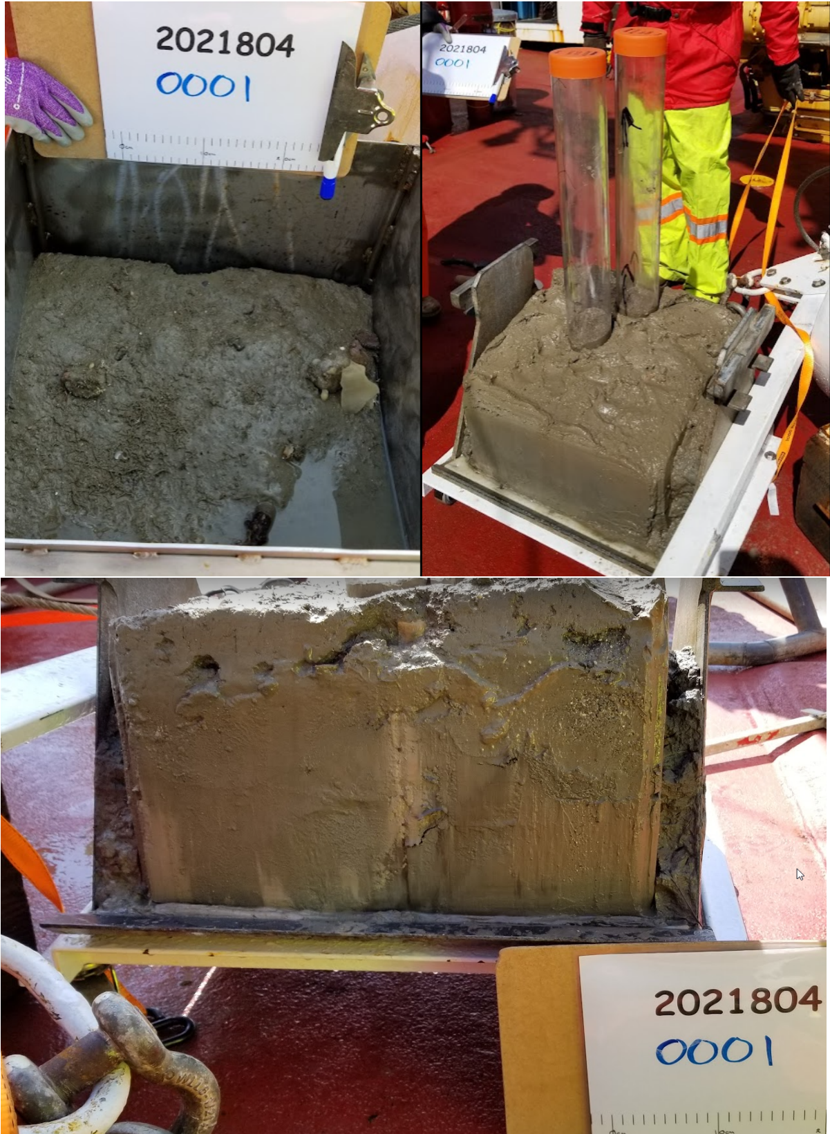
Figure 8 Surface, push cores and side view of the Box core sample. Photograph by V. Kostylev NRCAN photos 2021-507, 2021-508, 2021-509.
