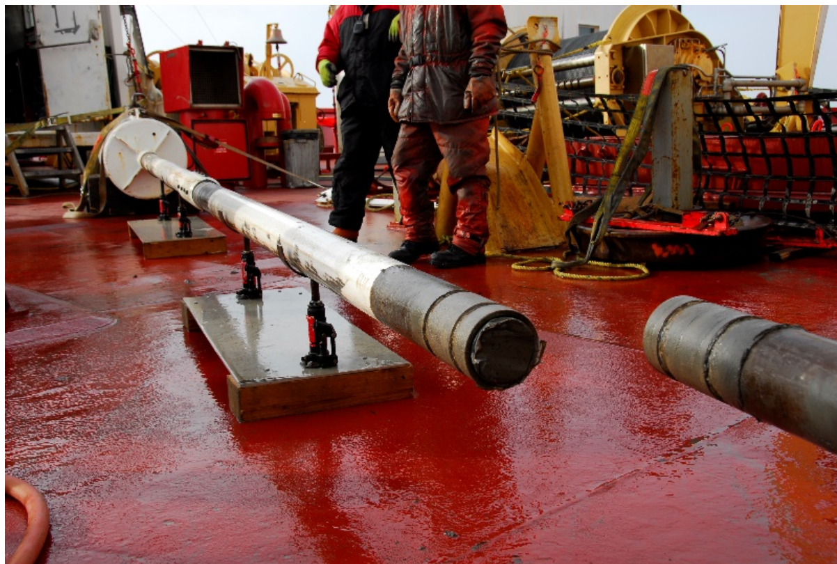
Figure 7. Piston core barrels separated on CCGS Amundsen forward deck, showing separated core liner. Photograph by V. Kostylev NRCAN photo 2021-506.
