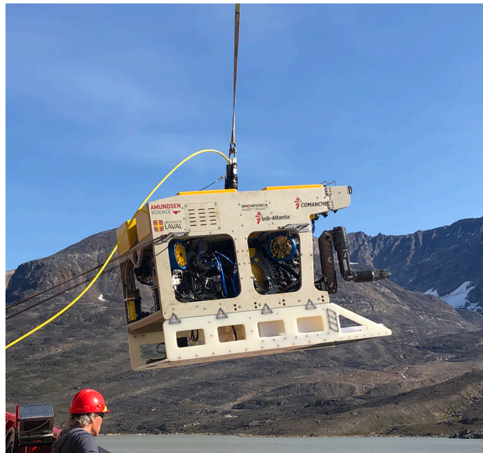
Figure 11: The Comanche ROV being deployed at Southwind Fjord. Photograph by A. Normandeau. NRCan photo 2021-262.
