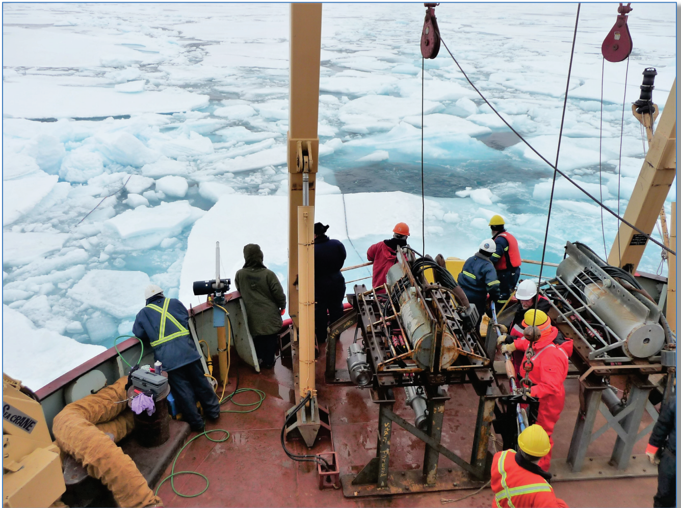
Figure 5: Deck crew and GSC technical staff carefully disentangling the hydrophone streamer from broken ice astern of the Canadian Coast Guard Ship Louis S. St-Laurent during the 2009 expedition. Photograph by J. Shimeld. NRCan photo 2021-494.
