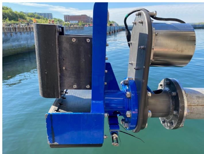
Figure 3: The R2Sonic 2022 multibeam echosounder on the R/V William-Kennedy pole. Photograph courtesy of Colin Gillies.
