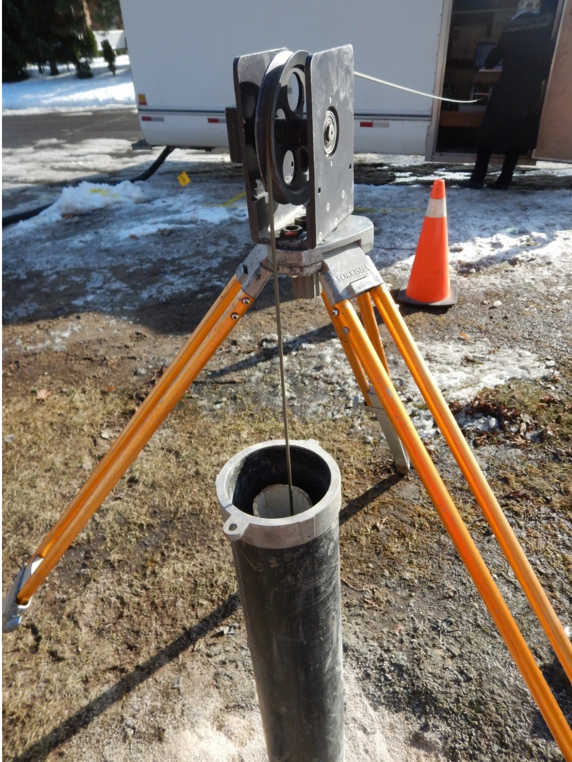
Figure 14. Geophysical logging of GSC-VC2; 3" PVC pipe is visible inside the ABS protective casing. Photograph by M.J. Hinton; NRCan photo 2022-336
