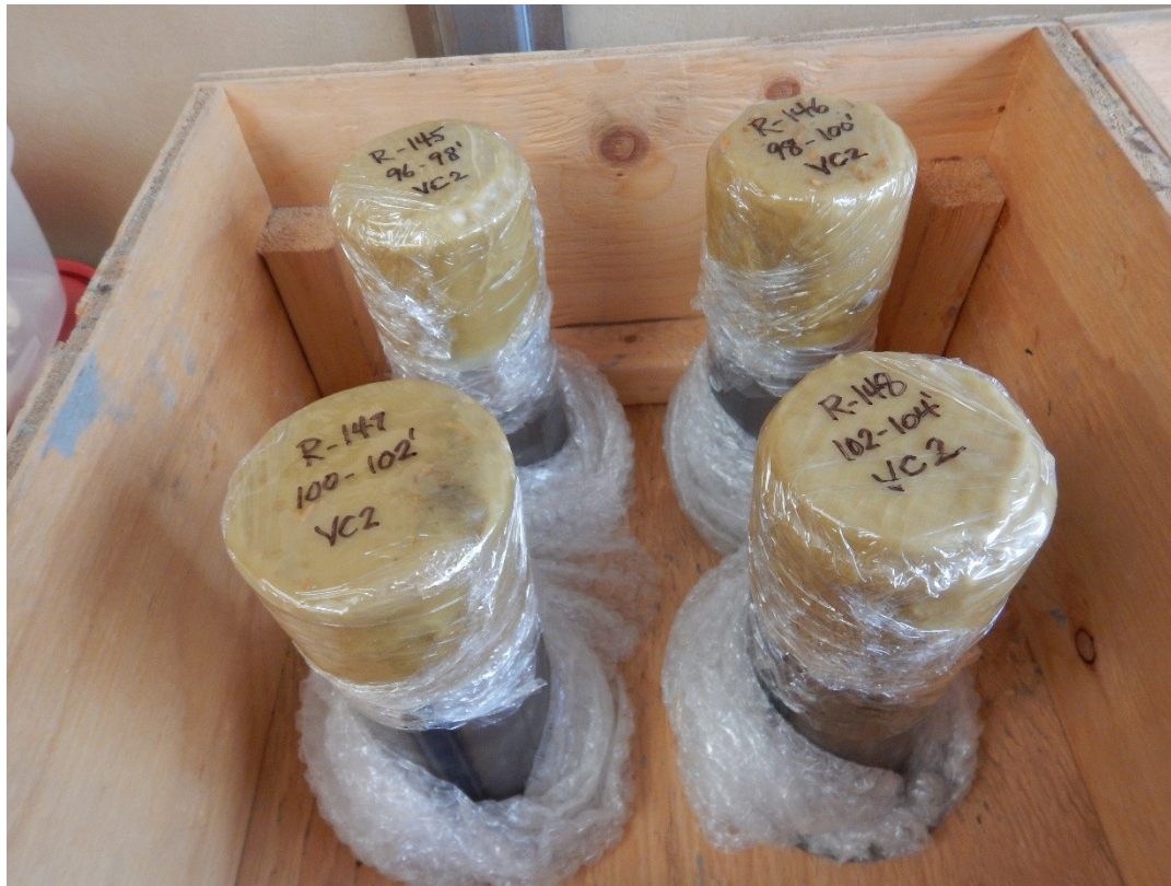
Figure 10. Cores sealed with wax mixture and packed for field transport to GSC; Photograph by M.J. Hinton, NRCan photo 2022-331
