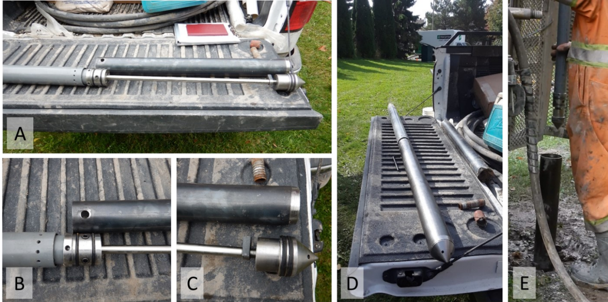
Figure 5. Piston corer; A) Piston in retracted position; B) Moveable piston head where Shelby tube attaches; C) Conical point; D) Shelby tube attached to piston corer, ready for deployment; and E) Piston extended and Shelby tube removed after sampling; Photographs A-C, E by M.J. Hinton, NRCan photos 2022-322 2022-323, 2022-324, and 2022-326 respectively; Photograph D by H.L. Crow, NRCan photo 2022-325
