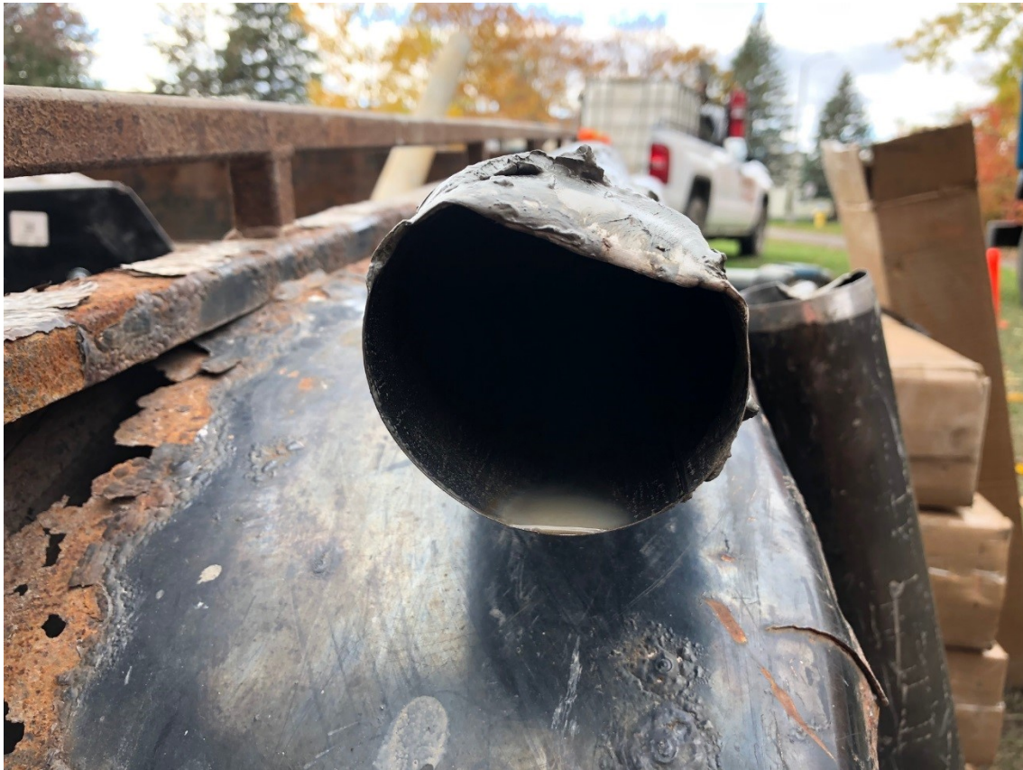
Figure 23. Shelby tube dented by a concretion; Photograph by M.J. Hinton, NRCan photo 2022-342
