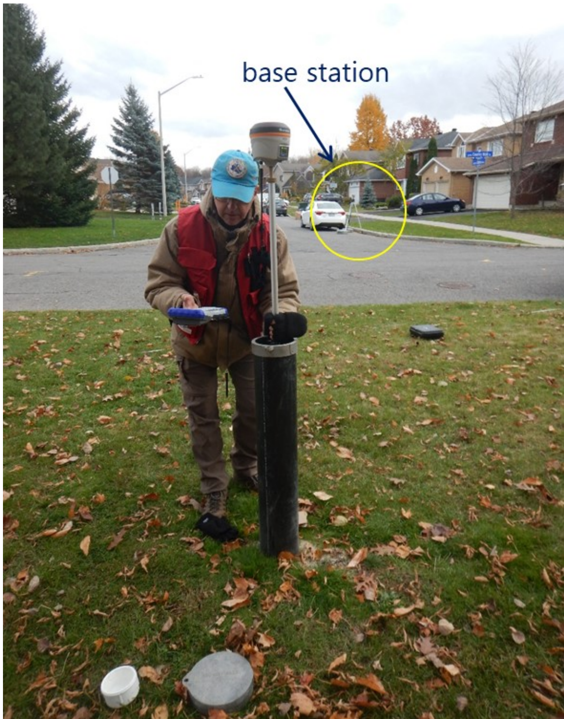
Figure 35. GPS survey of GSC-VC2 with the rover in the foreground and the base station in the background; photograph by M.J. Hinton, NRCan photo 2022-350.
