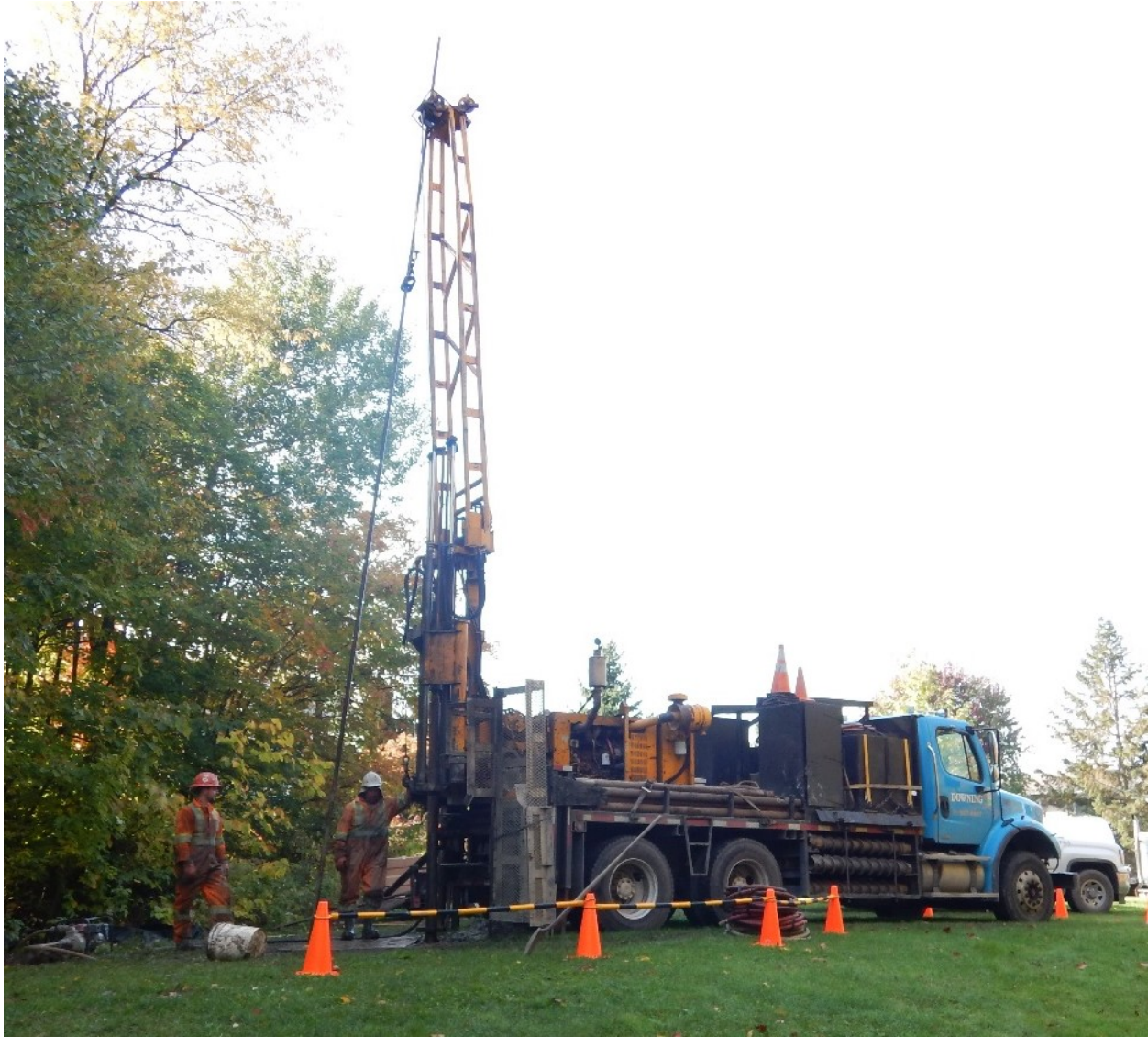
Figure 3. CME 75 drill rig at site BC16; Photograph by M.J. Hinton, NRCan photo 2022-321
