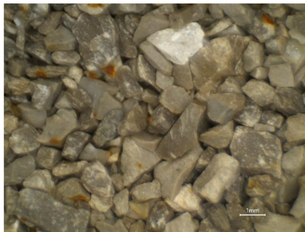
Figure 7. Dundee Formation drill cuttings from Norfolk County, Charlotteville Township (T002283), at a depth of 59.7m (196ft) (10x magnification). Photo courtesy of Alex Cachunjua.
