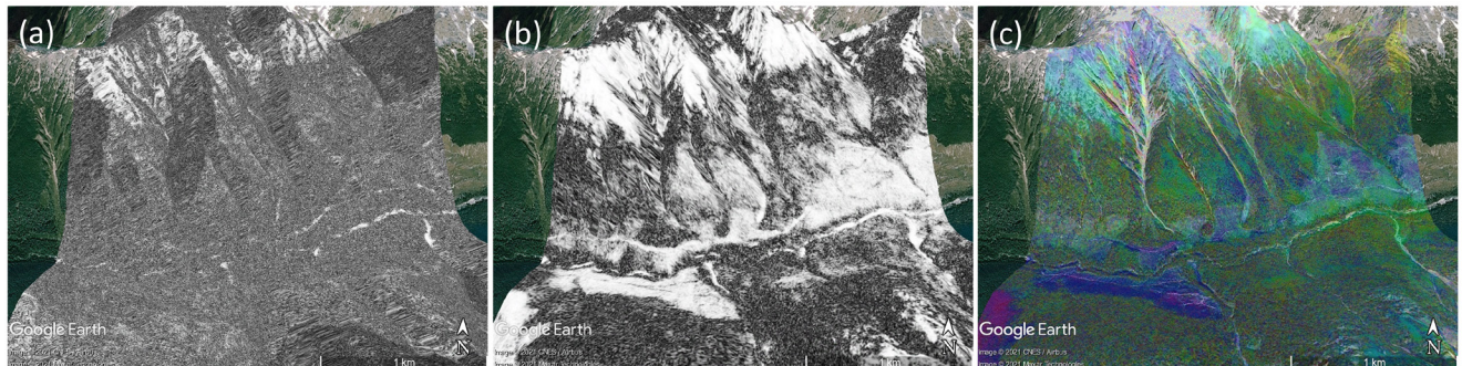
Figure 13. (a) RADARSAT-2 (U1) coherence of 20200529-20200622. (b) RCM (3M34) coherence of 20200524-20200528. (c) RCM (3M34) DInSAR interferogram of 20200524-20200528.
