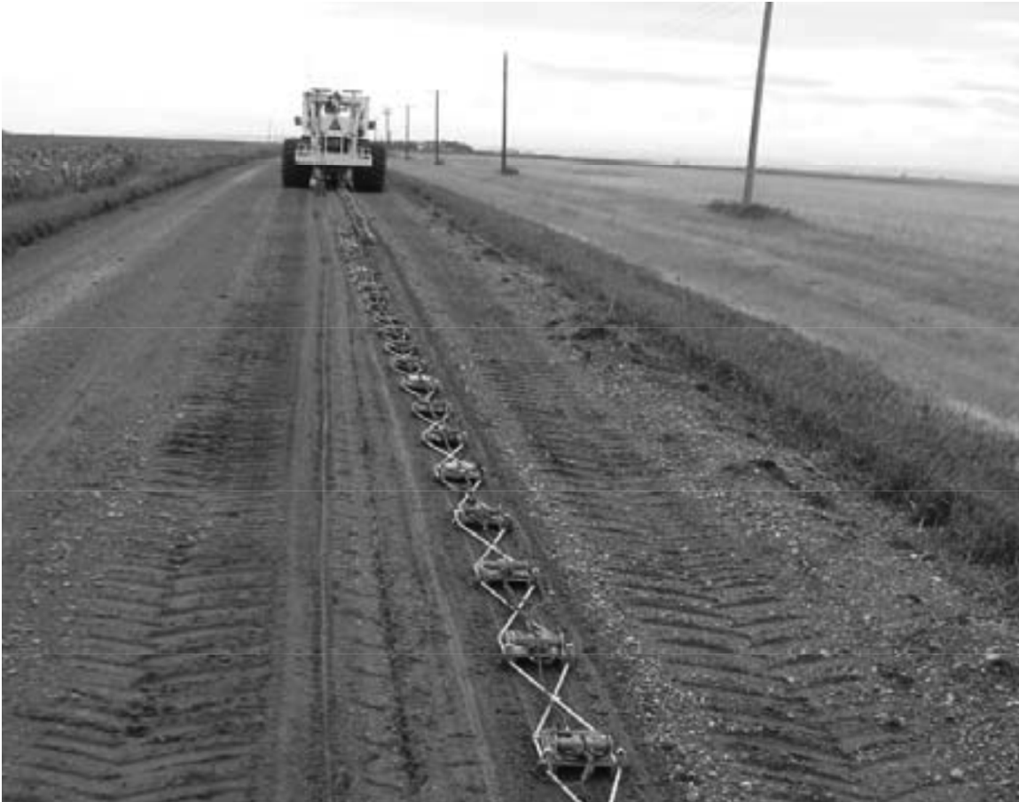
Figure 2: Photograph of the minivib source and SH-wave landstreamer in operation. Courtesy of Shawn Slattery.
