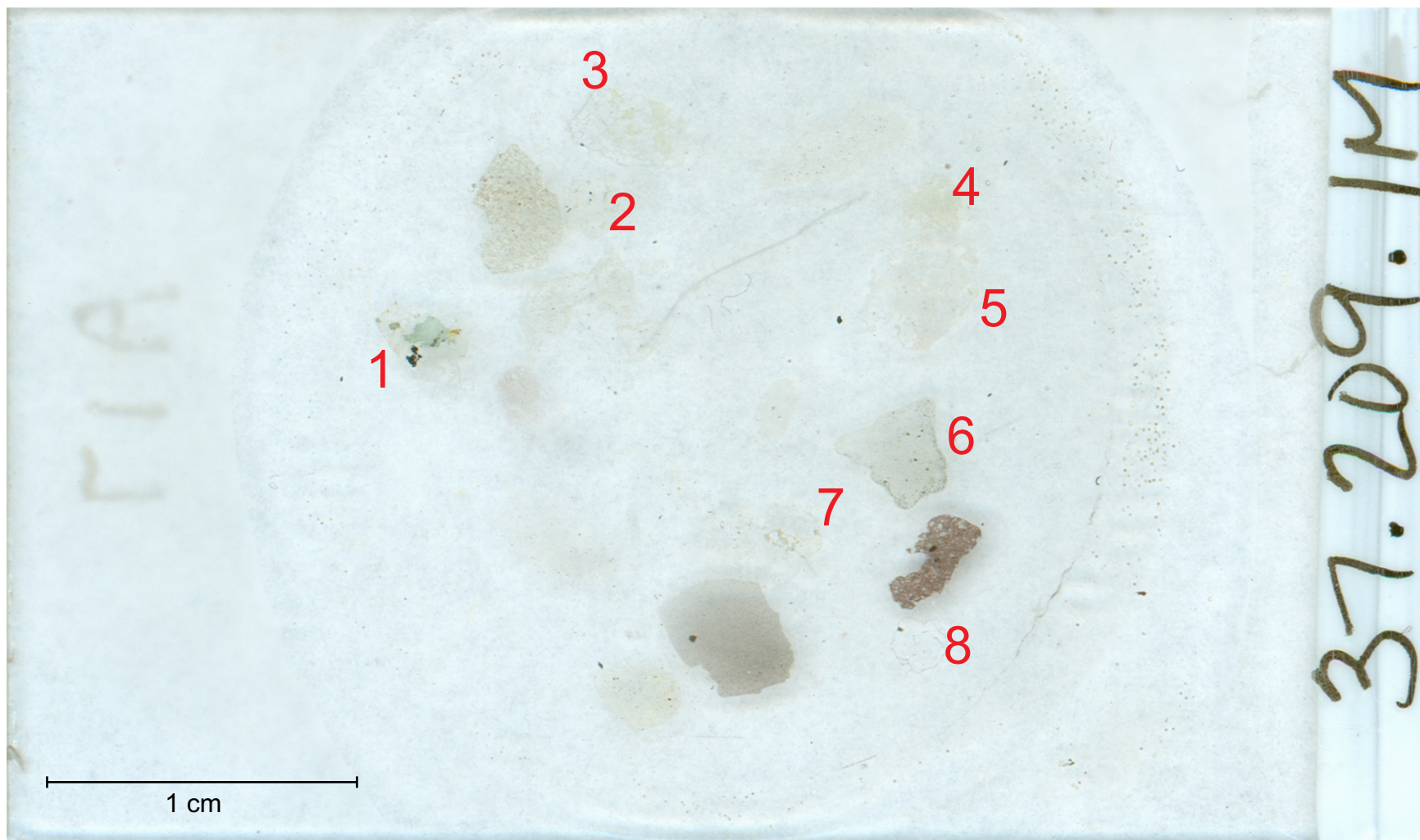
Figure 1-3A.1: Scanned thin section of Flemish Cap sample 217.1M. Granules are numbered in red corresponding to analysed sites.
