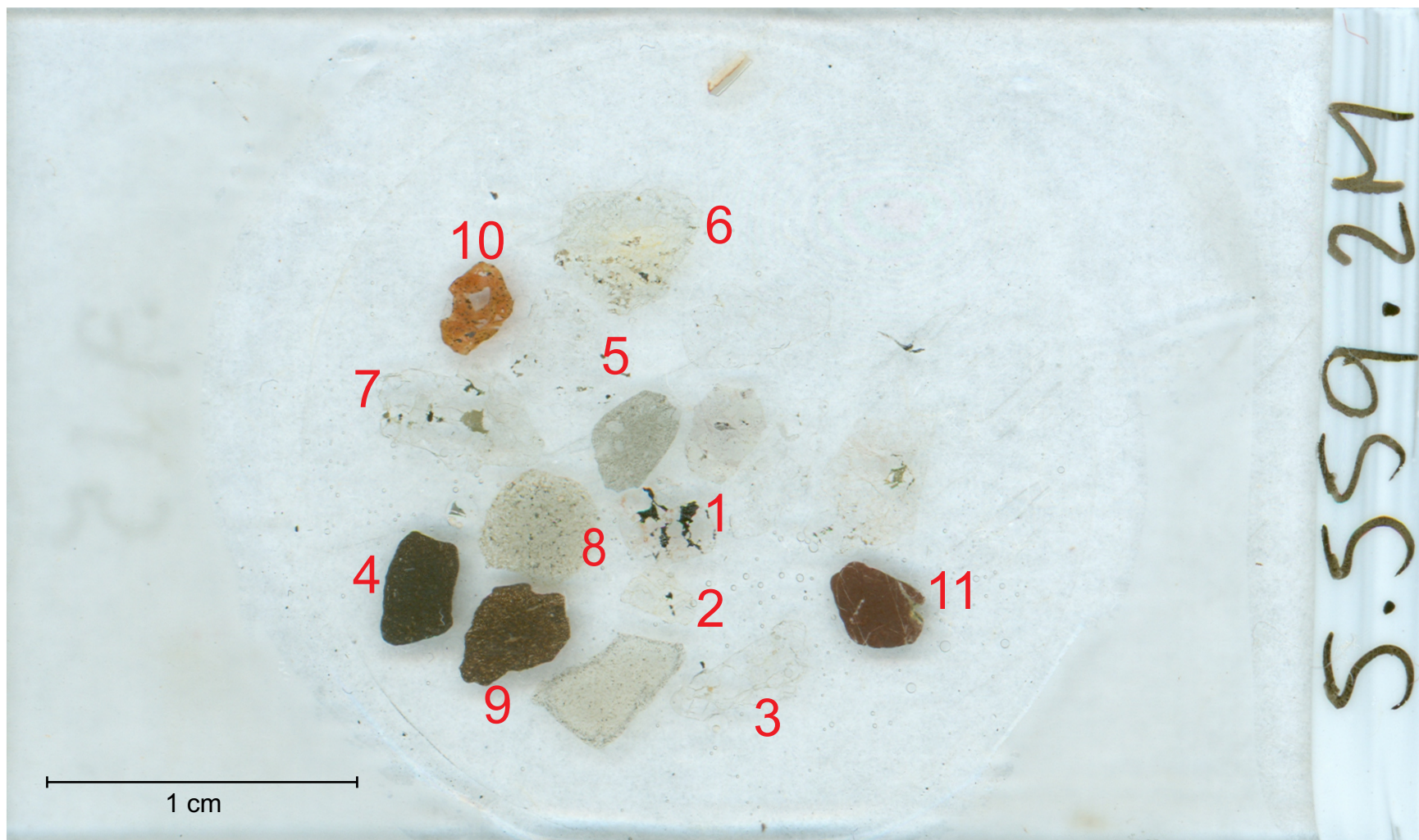
Figure 1-1B.1: Scanned thin section of Flemish Cap sample 195.2M. Granules are numbered in red corresponding to analysed sites.
