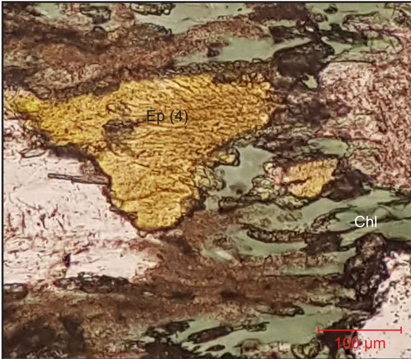
Figure 1-4A.48: Microphotograph. Sample 216.1L. Granule 2. Transmitted light, ppl, 10x. Site checked for presence of garnet but presence of epidote was confirmed.
