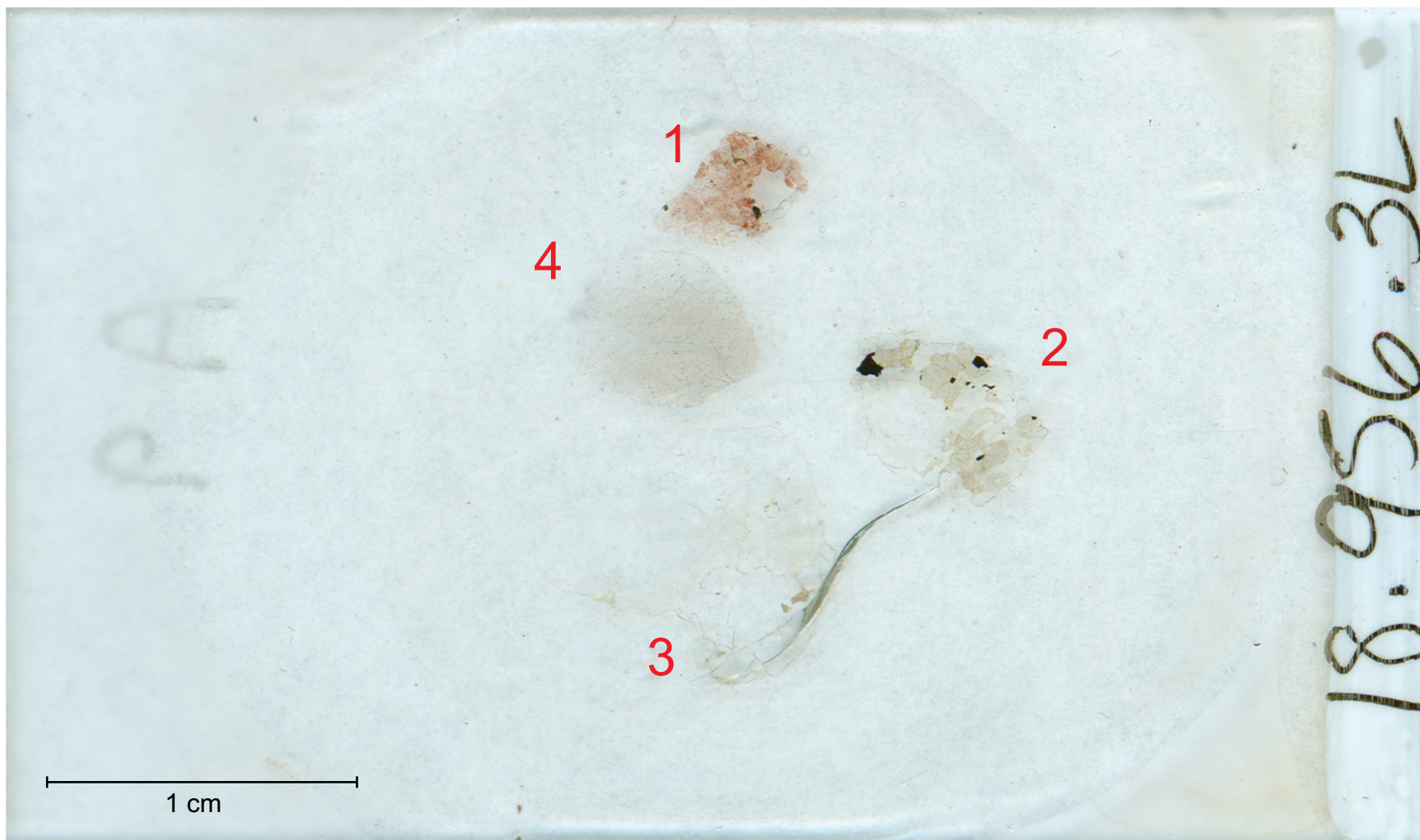
Figure 1-2B.1: Scanned thin section of Flemish Cap sample 229.3L. Granules are numbered in red corresponding to analysed sites.
