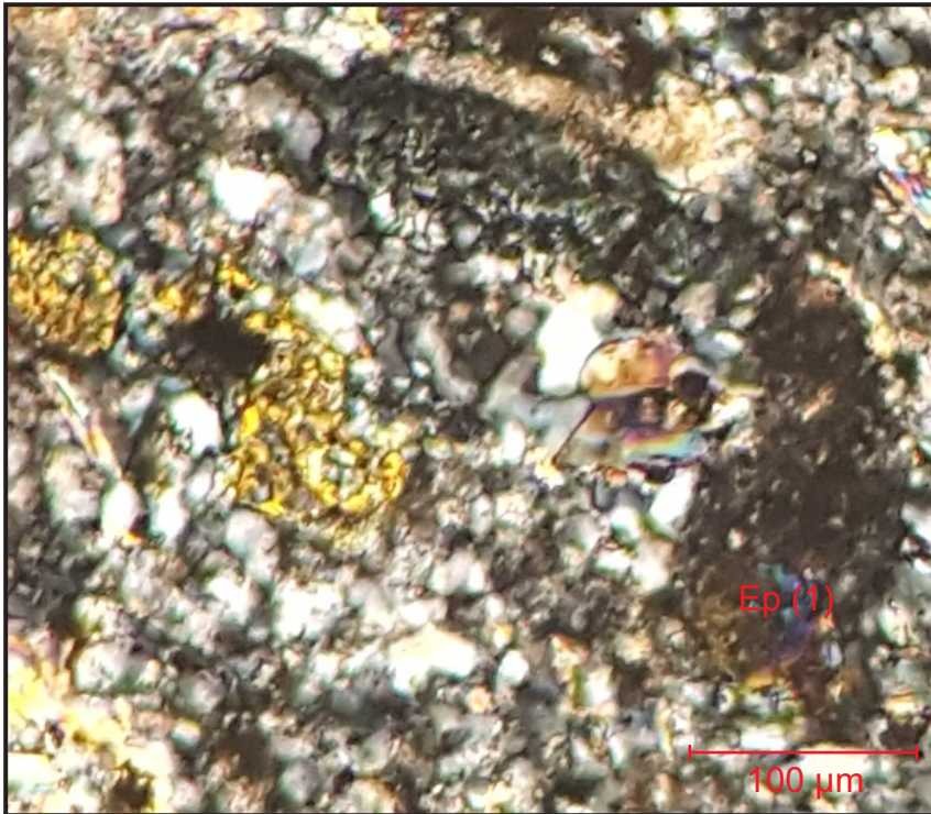
Figure 1-4A.52: Microphotograph. Sample 216.1L. Granule Site 8, Position 1. Transmitted light, ppl, 10x. The epidote analysed displays second order birefringence. Altered granitoid rock.
