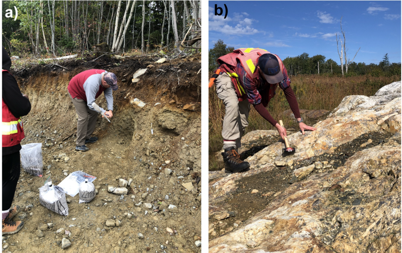
Figure 5. a) Collecting samples from a vertical till section for matrix geochemistry and indicator mineral analysis (Photograph by M.B. McClenaghan. NRCan photo 2022-575); b) collecting a bedrock sample for recovery of indicator minerals at the North pegmatite (Photograph by M.B. McClenaghan. NRCan photo 2022-576).
