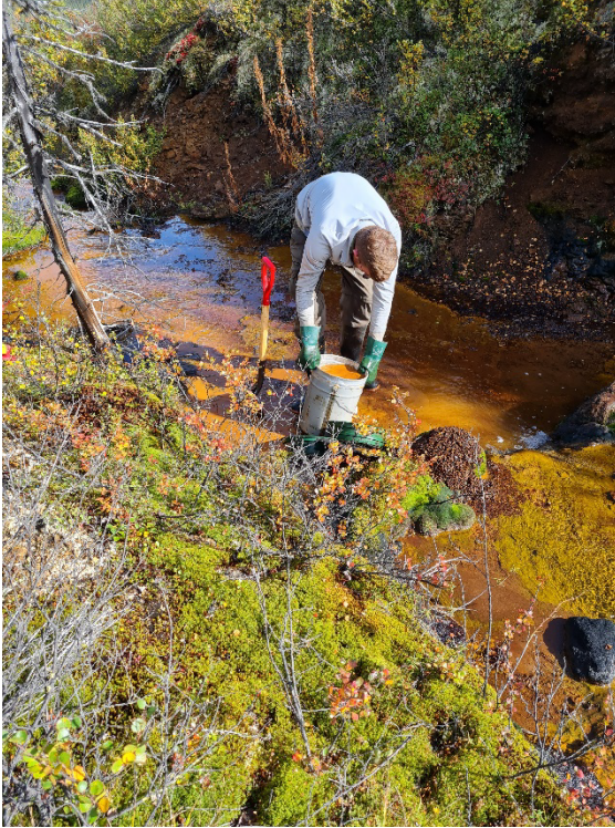
Figure 3: Collection of a bulk stream sediment (12 kg) sample in Proctor Gulch at site 115J221032. The bulk sample was sieved into a 20 L (5 gallon) pail lined with a labelled plastic sample bag in order to recover the <2 mm fraction for heavy mineral analysis. Water is drained from the sample bag after sufficient sample material has been collected and before closing the sample bag. Photograph by J.E. Kidder. NRCan Photo 2022-450.
