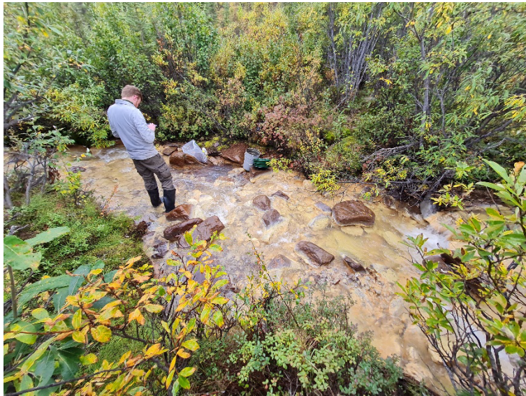
Figure 2: GSC geologist Chris Beckett-Brown logging site field data on the tablet after collecting stream sediment samples at site 115J221030 near the Casino deposit. Note the pale white precipitate on the stream bed, which is suspected to be an Al-sulfate. Photograph by J.E. Kidder. NRCan Photo 2022-449.
