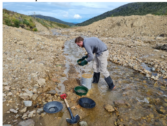
Figure 4: An example of GSC geologist Chris Beckett-Brown separating the 2-10 mm clast fraction at sample site 115J221004 following wet sieving the bulk stream sediment sample into the plastic sample bag lined pail. Photograph by J.E. Kidder. NRCan Photo 2022-451.
