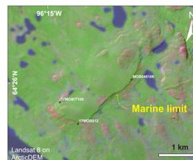
Trimline at 118 m elevation west of Baker Lake. Thick glacial sediments are found above the marine limit; reworked sediments and bedrock outcrops occur below the limit of marine inundation.
