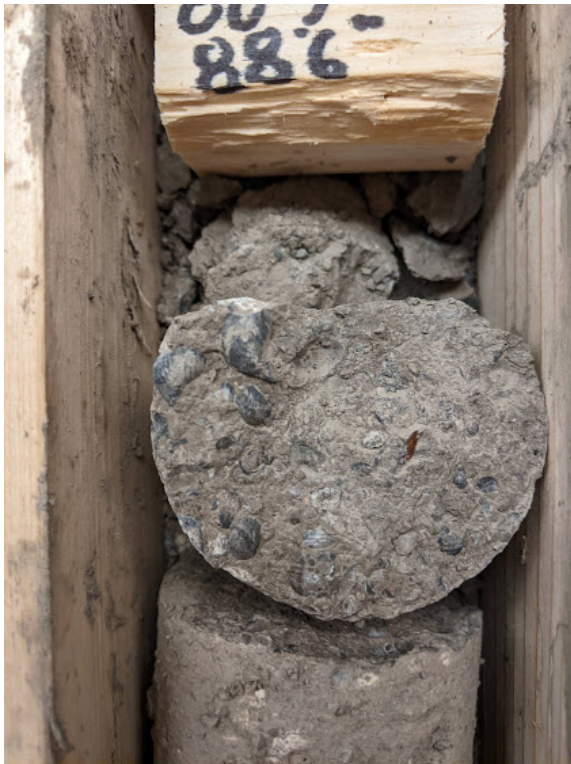
Photo at 28.8 m. Fine-grained sandstone with bivalves and gastropods.
