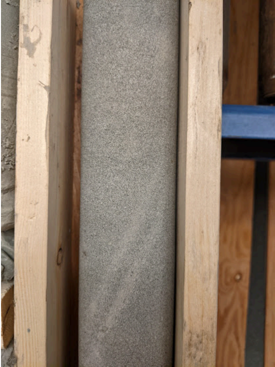
Photo at 23 m. Medium-grained calcareous sandstone.
