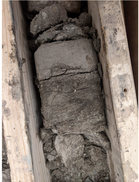
Photo at 26.5 m. Mudstone with coal laminae.
