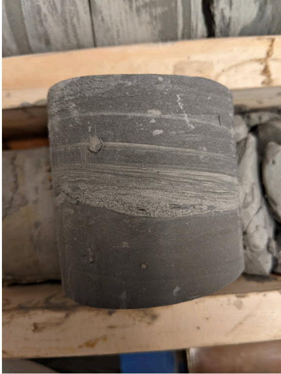
Photo at 39 m. Small channel filled sandstone in mudstone.
