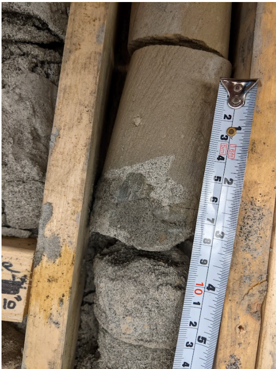
Photo at 66.2 m. Compaction-driven injection of sandstone in mudstone.
