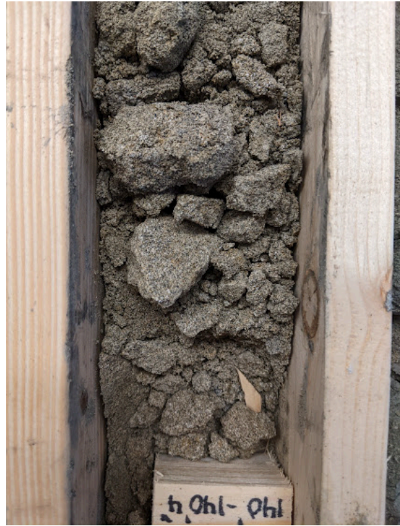
Photo at 42.7 m. Very friable calcareous coarse sandstone.
