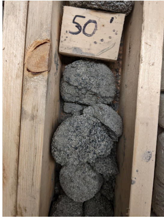
Photo at 15.2 m. Friable calcareous sandstone.
