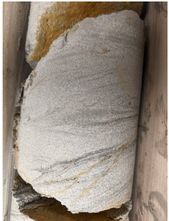
Photo at 31.4 m. Cross-laminated fine grained sandstone.
