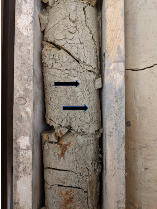
Photo at 15.8 m. Soil slickensides (arrows).
