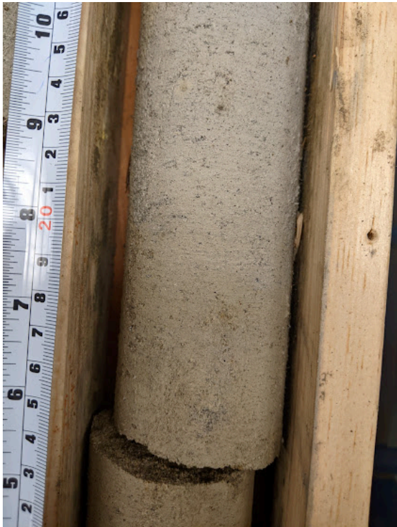
Photo at 55.8 m. Calcareous fine-grained sandstone.
