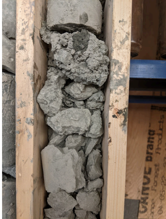
Photo at 31.5 m. Fine-grained friable calcareous sandstone.
