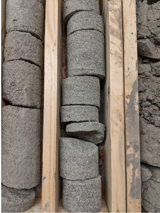
Photo at 13.4 m. Calcareous coarse-grained sandstone.
