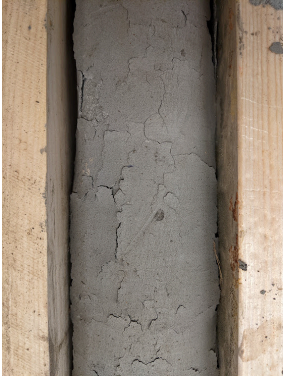
Photo at 25.3 m. Shale with clay shrinkage.
