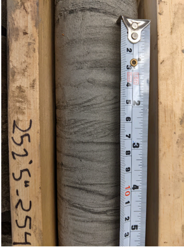
Photo at 79.2 m. Cross-laminated calcareous sandstone.
