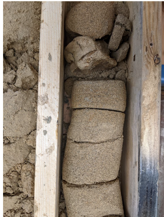
Photo at 29 m. Friable sandstone.
