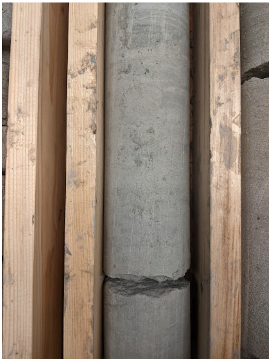
Photo at 20.6 m. Fine-grained sandstone.
