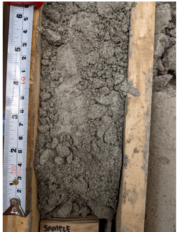
Photo at 62.1 m. Calcareous coarse-grained sand.
