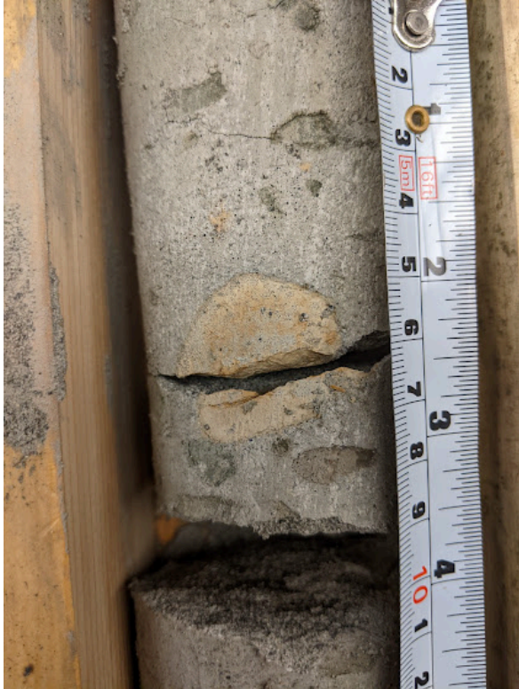
Photo at 65.2 m. Coarse-grained sandstone with mudstone clasts.
