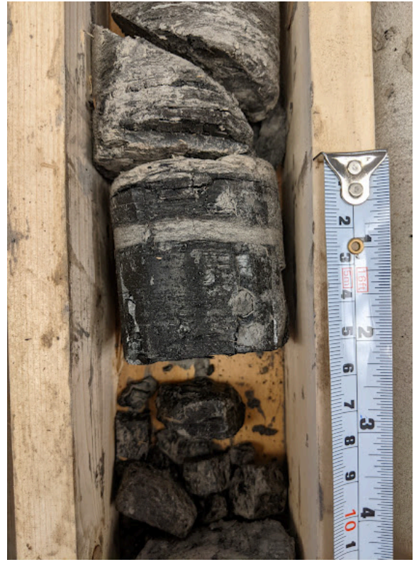
Photo at 83 m. Coal layer with siltstone interbeds.
