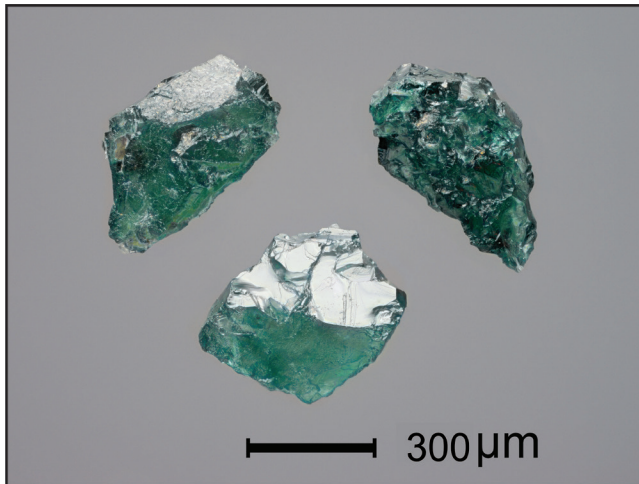
Figure 16. Colour photograph of blue-green, sand-sized gahnite grains used as an indicator mineral to map dispersal from the high-grade metamorphosed Izok Lake volcanogenic massive sulphide deposit, Nunavut. Photograph by Michael J. Bainbridge Photography.
