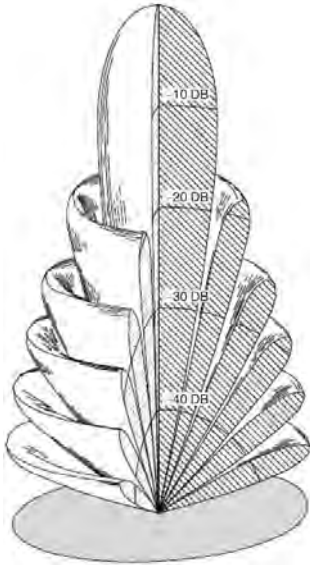
Figure 2. Typical 3-D beam pattern of a circular transducer (Massa 2003).
