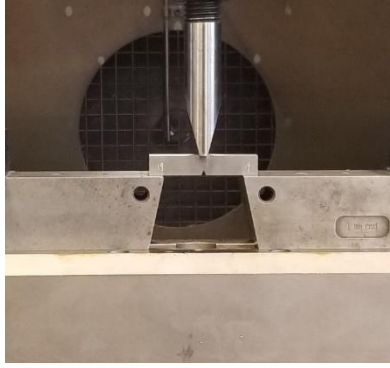
Figure 31: Static Charpy Sample Test fixture
