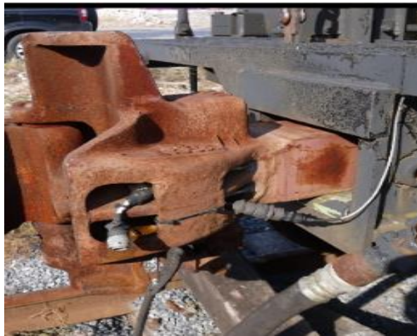
Figure 3: Instrumented coupler for measuring longitudinal coupler forces used by the FRA[10]
