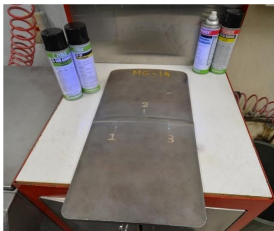
Figure 3 – Liquid penetrant inspection on defect specimen
