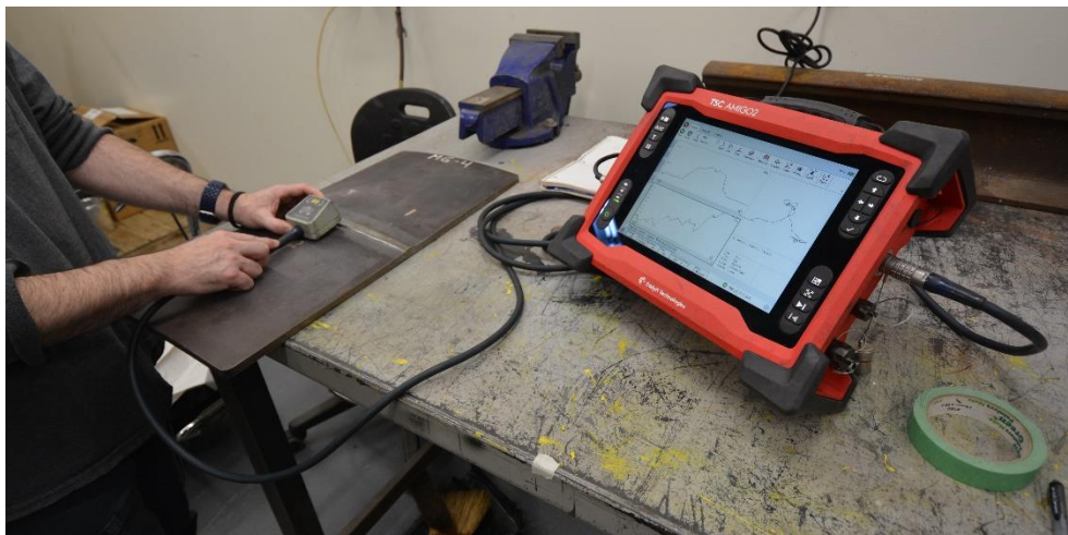
Figure 9 – ACFM inspection on defect specimen
