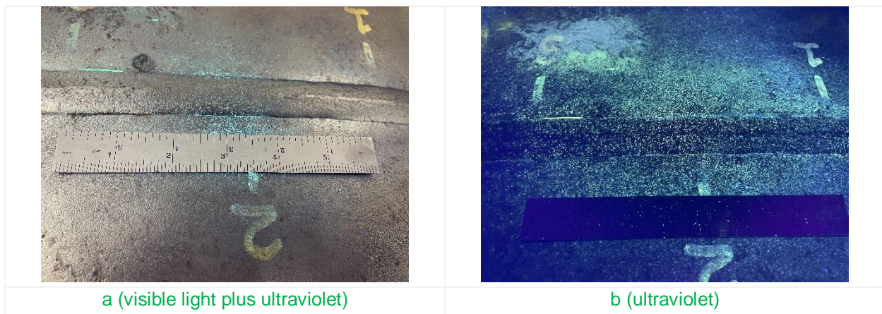
Figure 18 – PT indications of specimen MG-18 at location #2
