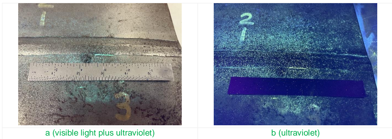
Figure 19 – PT indications of specimen MG-18 at location #3
