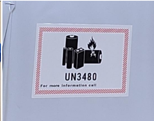
Figure 4: Box B4-1 internal packaging UN3480 label is missing a phone number
