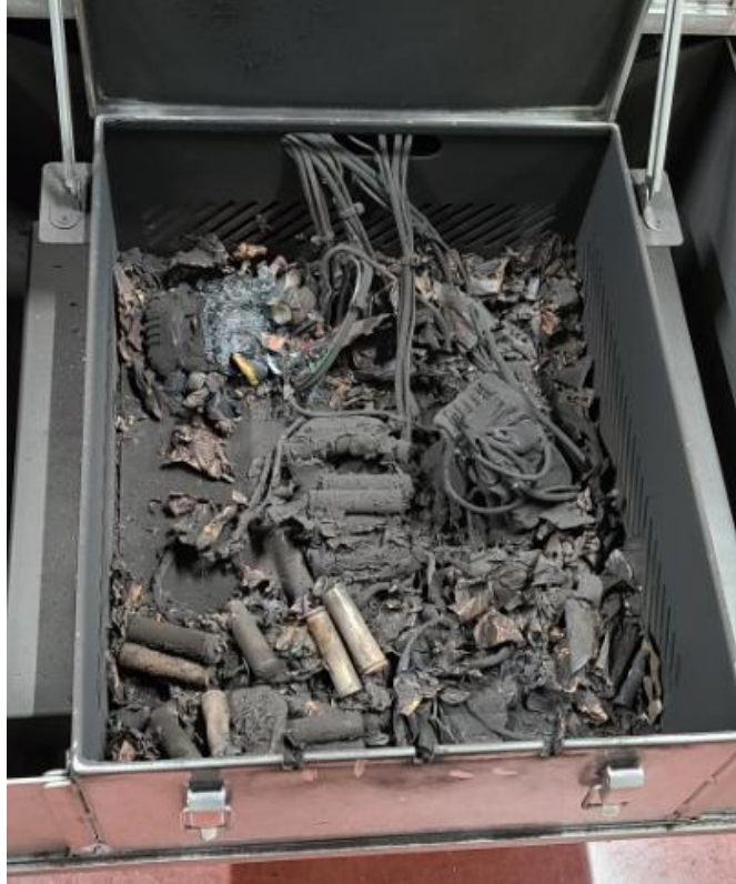
Figure 15: A4 Samples showing charring during the T.7 overcharge test
