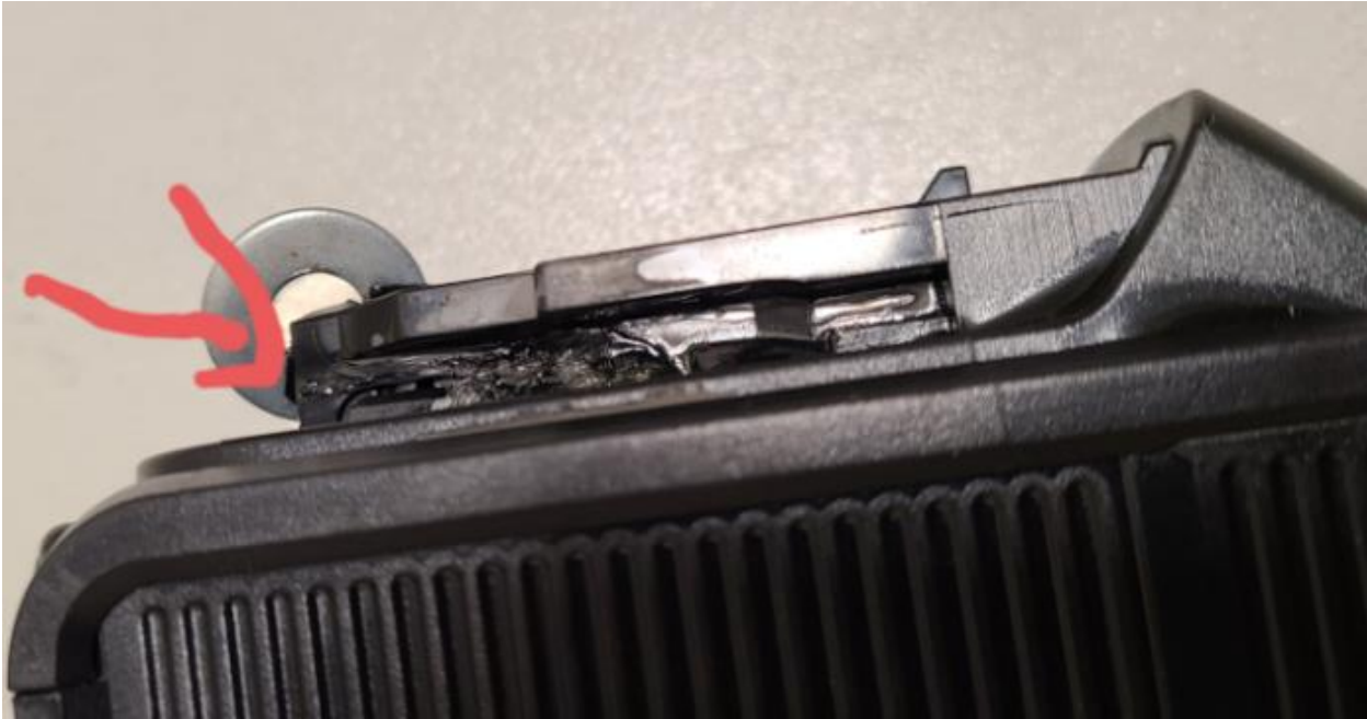
Figure 9: A2 Sample 5 T.5. - Melting of the plastic case due to the heat generated during the test
