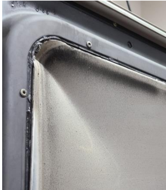
Figure 17: One A4 battery exploded with such force it dented the door of the explosion proof oven.
