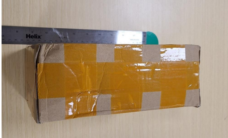
Figure 1: B6 Package (Box B6-1) is dented and appears to be retaped. Similar damage was observed for packages for A1, A3, A5, B1, B3, C1, C2, C3, C4, and C5.
