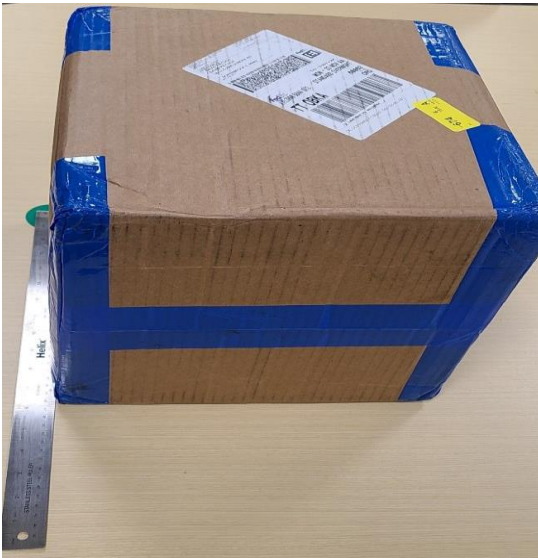
Figure 3: Box B4-1 Is missing a UN3480 label, only the pictured marking was available
