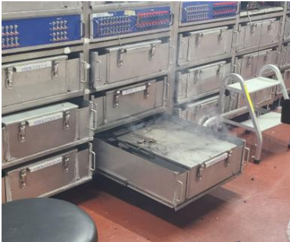
Figure 14: A4 Samples releasing a heavy amount of smoke after catching fire and exploding during the T.7 overcharge test
