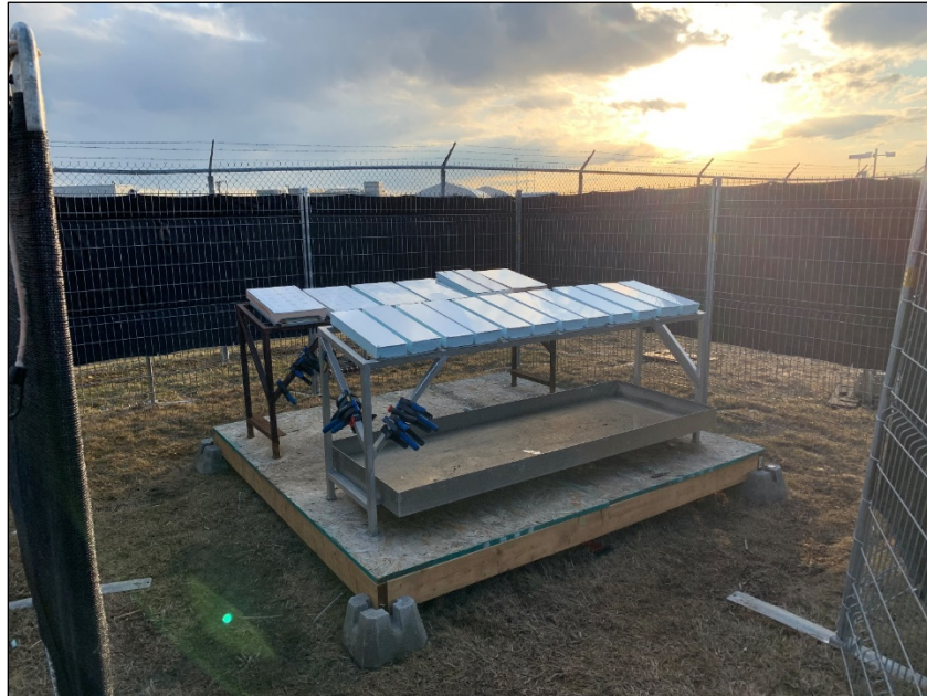
Photo 2.1: Test Stand Installed Inside the DFIR Shield
