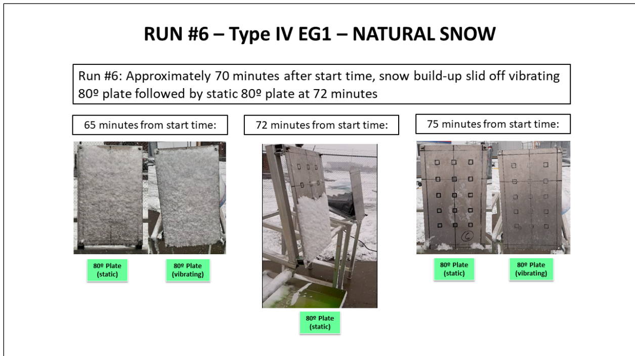
Figure 5.10: Run #6 – Vertical Plates Snow Build-Up Run-Off
