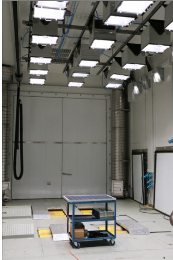
Photo 16.1: Large Climate Chamber at the ACE Facility
