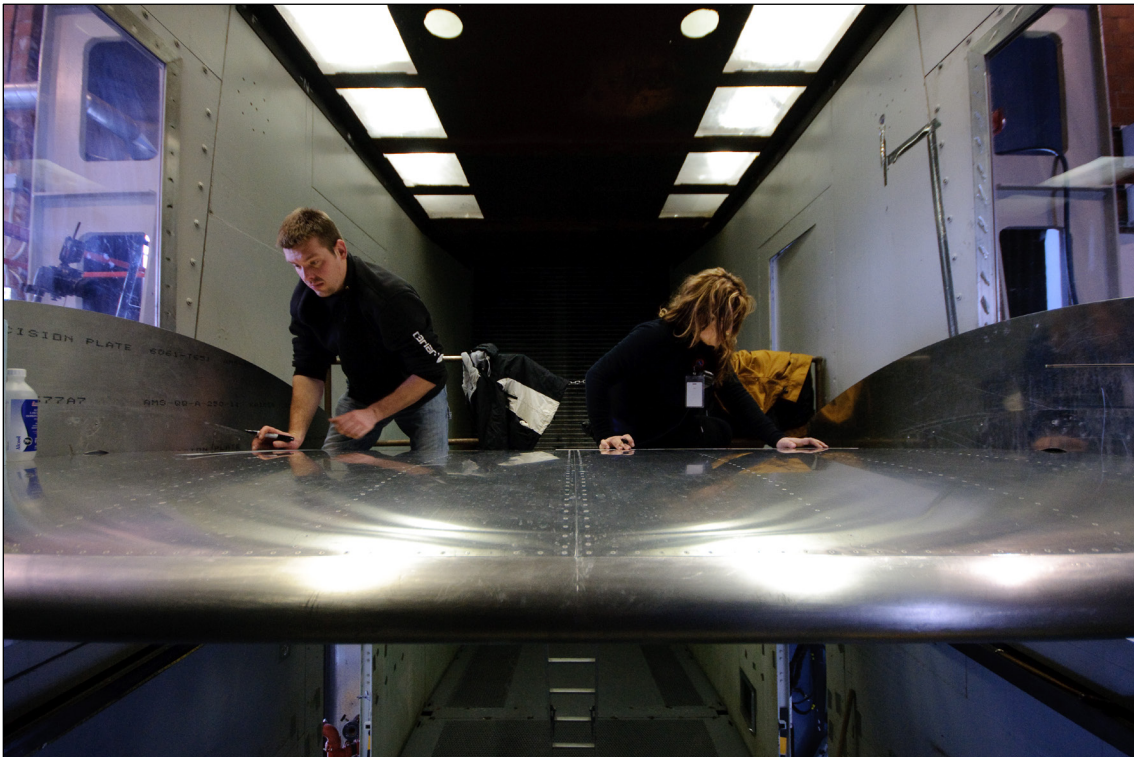
Photo 2.3: Thin High-Performance Wing Section Used for Testing
