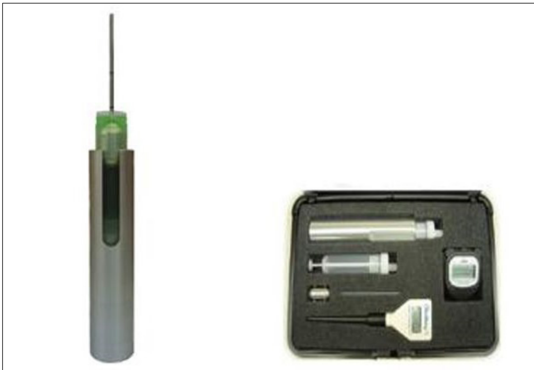
Photo 2.14: Stony Brook PDVdi-120 Falling Ball Viscometer
