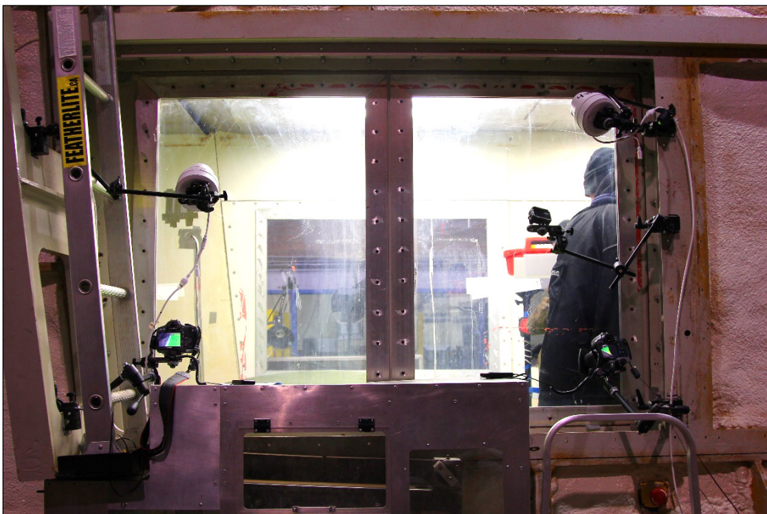
Photo 2.10: Wind Tunnel Setup for Digital Cameras
