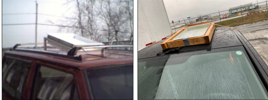
Photo 5.1: Example Images of a Rate Pan Installed on a Test Vehicle
