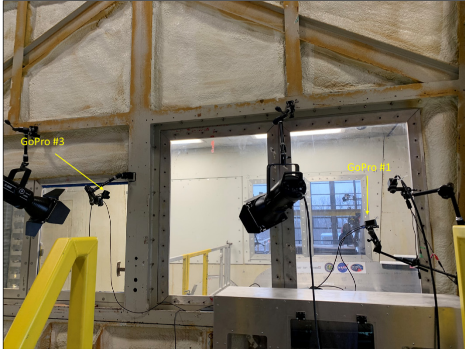
Figure 5.2: Location of Cameras – North Side of Wind Tunnel During RJ Wing Testing
