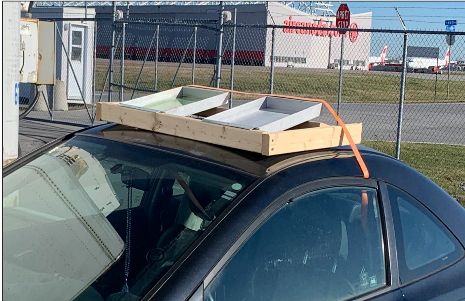
Photo 3.1: Method 1 – Simulated Taxiing Aircraft
