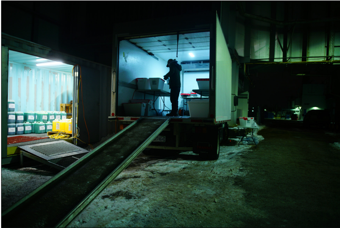
Photo 2.5: Refrigerated Truck Used for Manufacturing Ice Pellets
