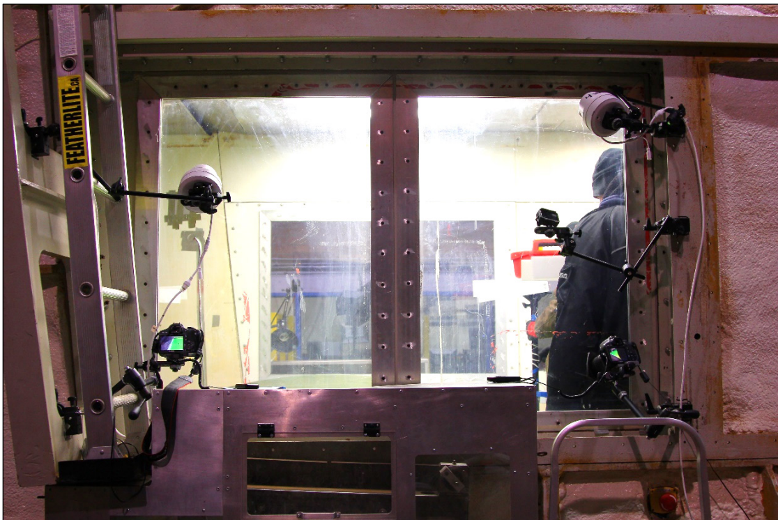
Photo 2.10: Wind Tunnel Setup for Digital Cameras
