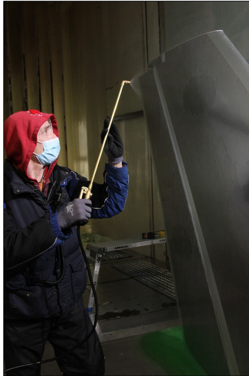
Photo 2.9: Simulating Freezing Rain with Garden Sprayer
