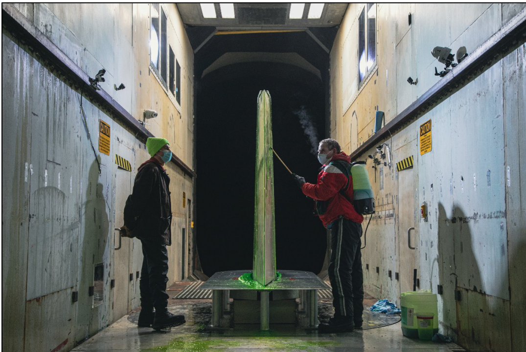
Photo 2.4: Vertical Stabilizer Mounted in the NRC IWT for Testing
