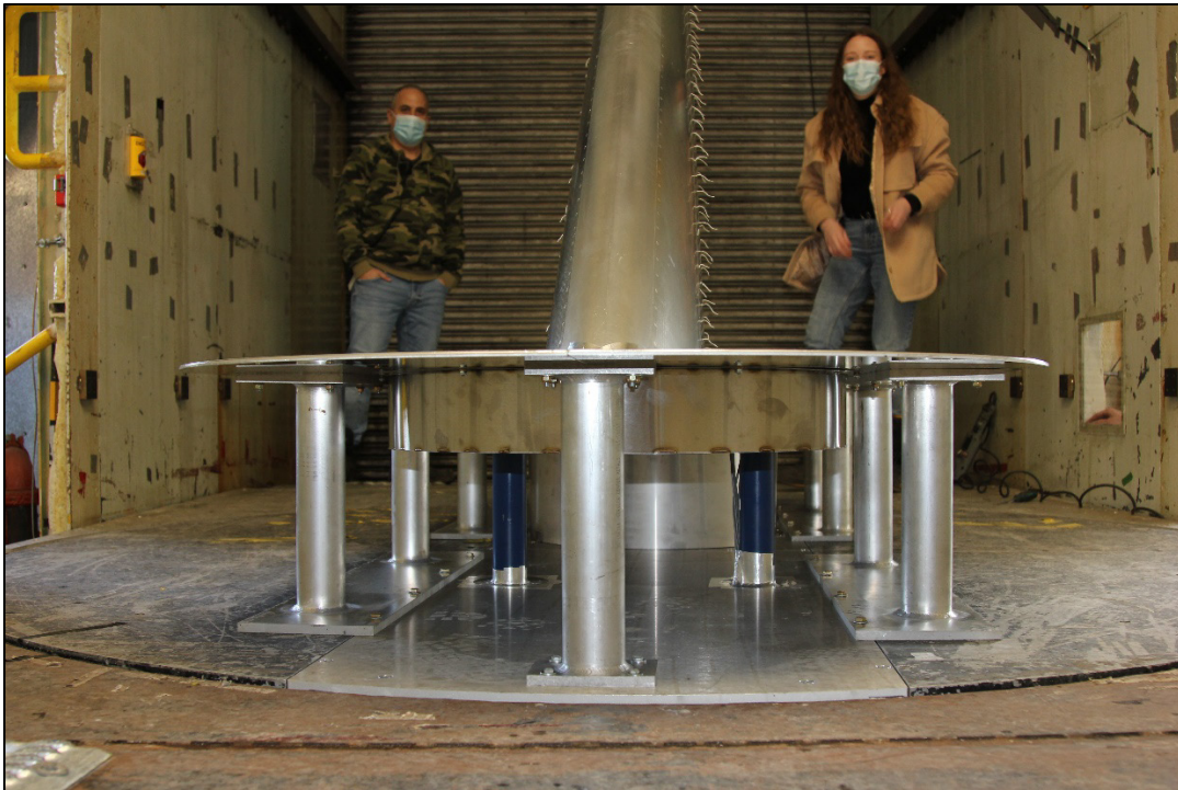
Photo 2.5: View of Splitter Plate Used to Mount the CRM
