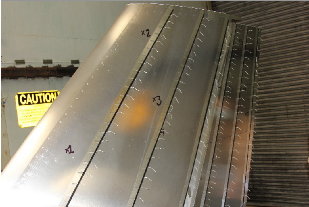
Photo 5.1: Tufts Attached to the Vertical Stabilizer Model Using Speed Tape
