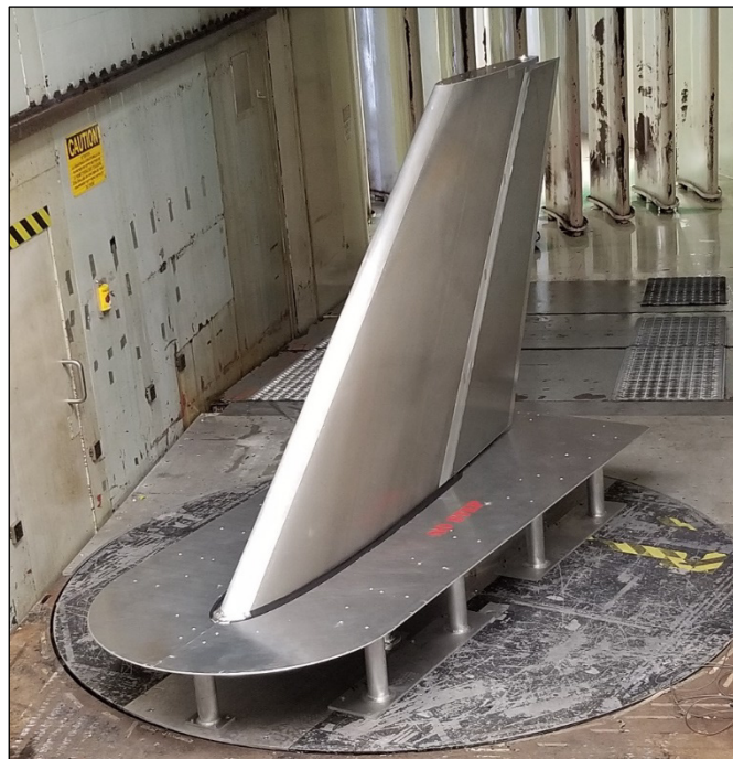
Photo 2.2: Inside View of the NRC Icing Wind Tunnel Test Section with CRM
