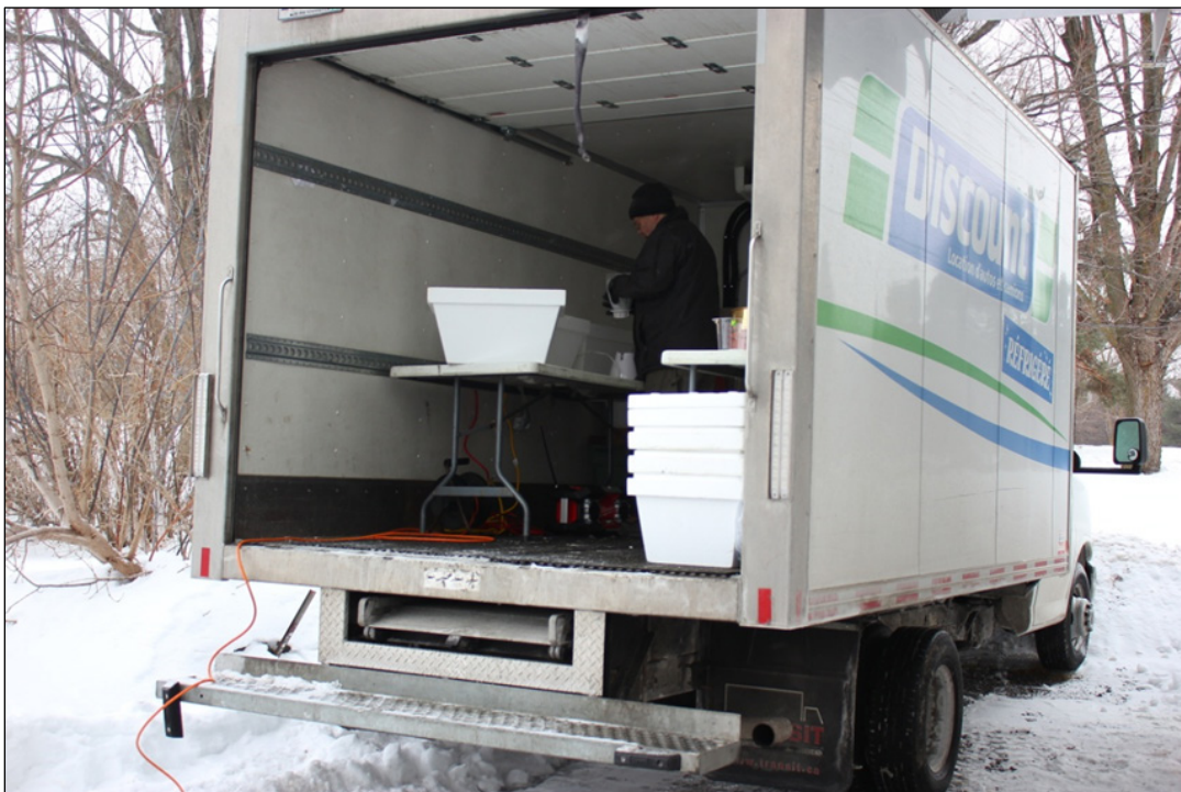
Photo 2.6: Refrigerated Truck Used for Manufacturing Ice Pellets
