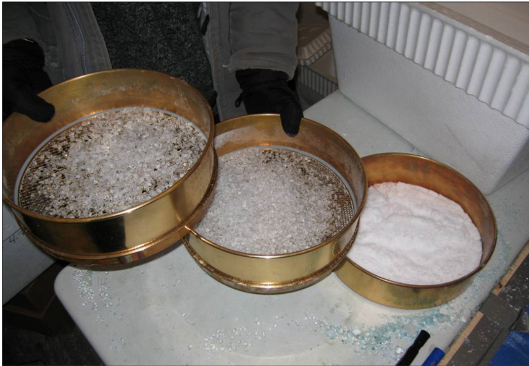
Photo 2.7: Calibrated Sieves Used to Obtain Desired Size Distribution
