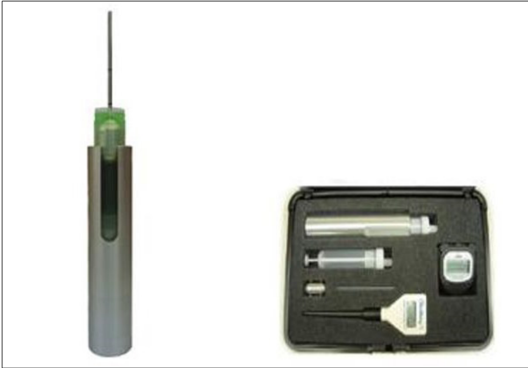
Photo 2.15: Stony Brook PDVdi-120 Falling Ball Viscometer
