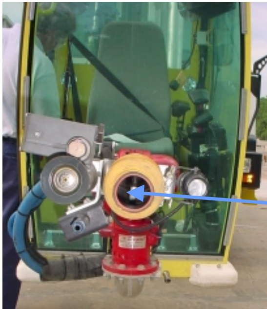
Photo 2.2: Detail of Fluid Injection Nozzle used by FedEx (shown with a variety of nozzles available for FMC forced air system)
