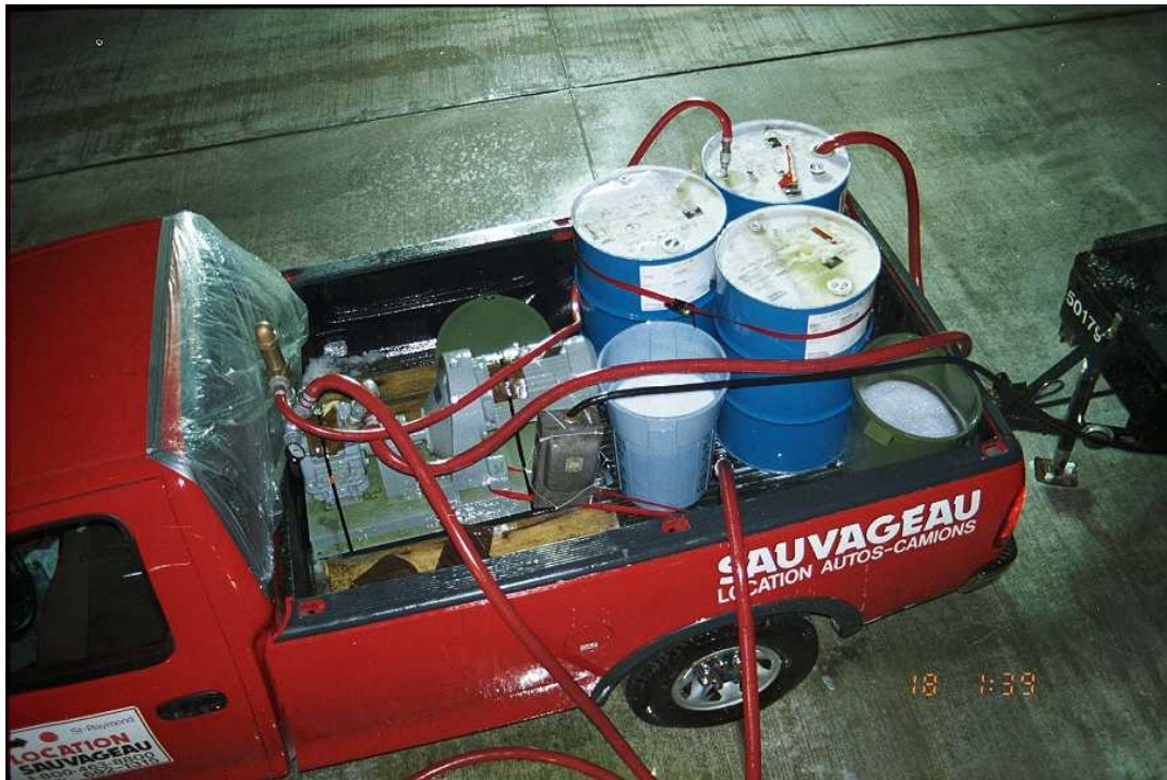
Photo 2.7: Mobile Type IV Fluid Sprayer Unit
