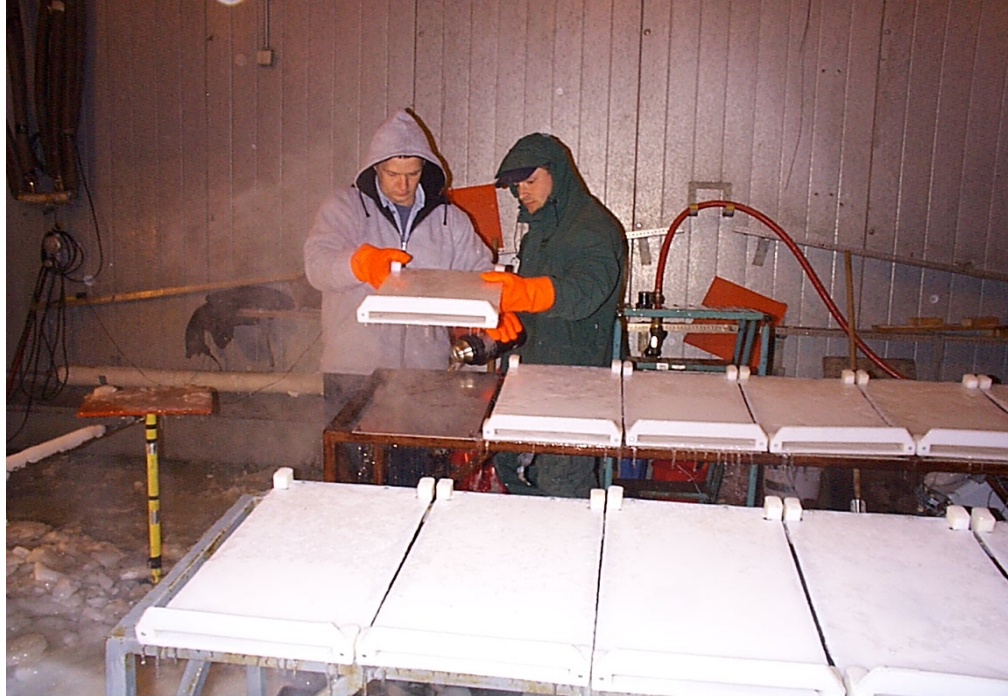
Photo 2.17: Pouring of Type IV Fluid While Plate is Covered to Protect from Precipitation
