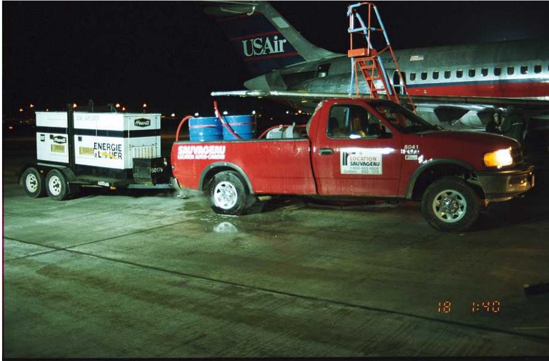
Photo 2.9: Type IV Mobile Sprayer Set-up
