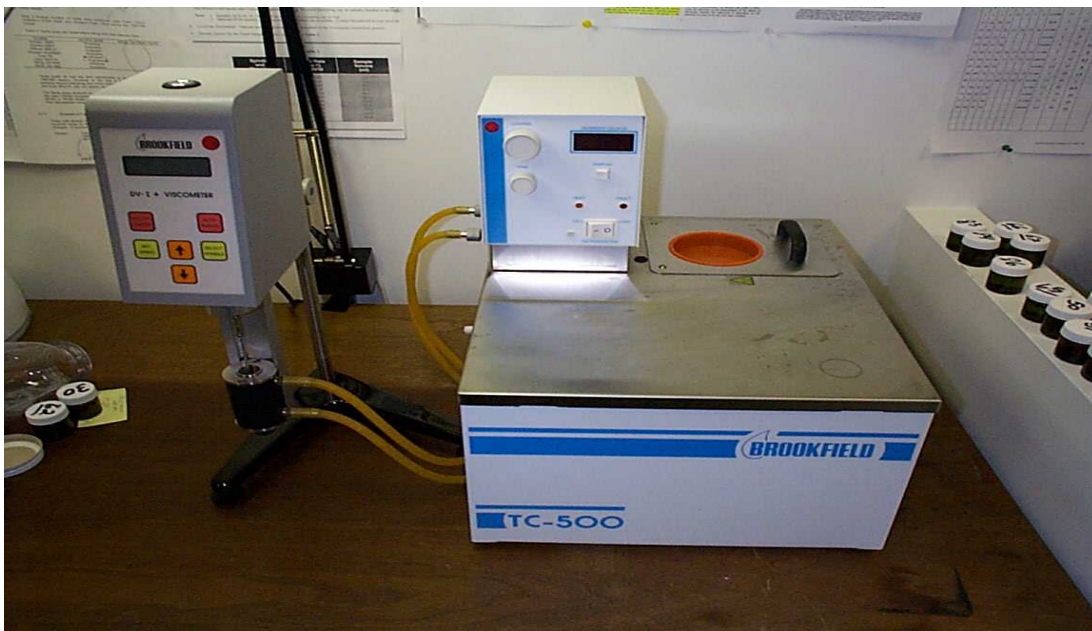
Photo 2.10: Brookfield Digital Viscometer Model DV-I+ and Temperature Bath
